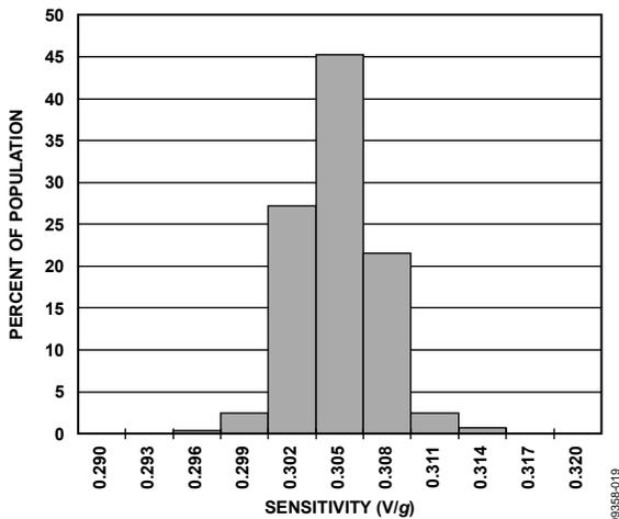
Figure 17. Z-Axis Sensitivity at 25°C, V<sub>S</sub> = 3 V
