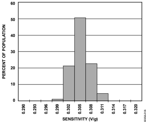
Figure 16. Y-Axis Sensitivity at 25°C, V<sub>S</sub> = 3 V
