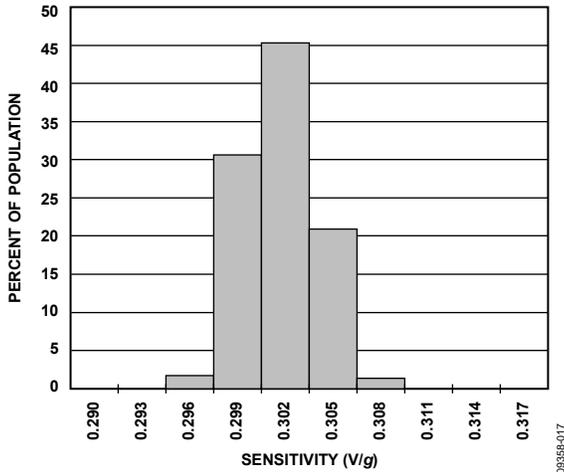
Figure 15. X-Axis Sensitivity at 25°C, V<sub>S</sub> = 3 V
