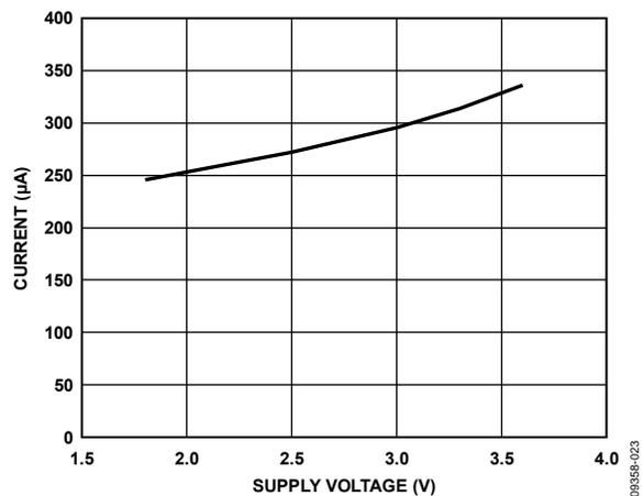
Figure 21. Typical Current Consumption vs. Supply Voltage
