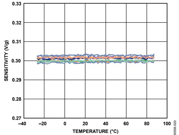
Figure 18. X-Axis Sensitivity vs. Temperature, Eight Parts Soldered to PCB, V<sub>S</sub> = 3 V
