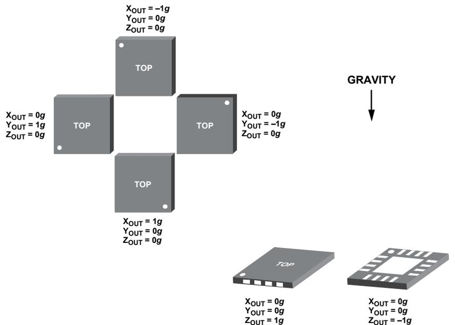
Figure 24. Output Response vs. Orientation to Gravity
