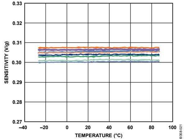
Figure 19. Y-Axis Sensitivity vs. Temperature, Eight Parts Soldered to PCB, V<sub>S</sub> = 3 V
