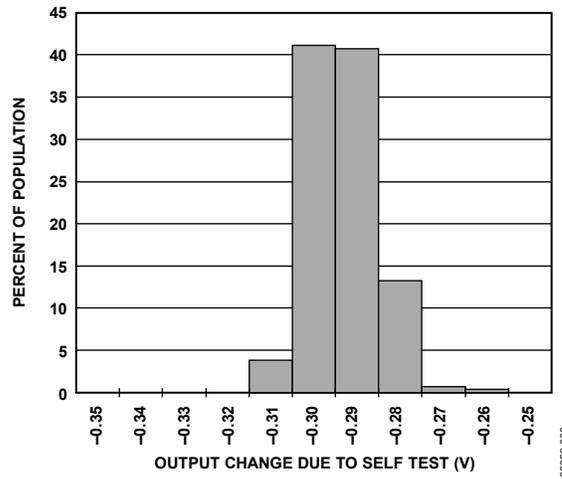
Figure 6. X-Axis Self-Test Response at 25°C,  $V_s = 3 V$
