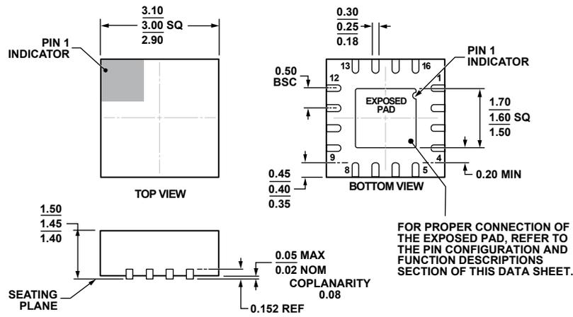
Figure 27. 16-Lead Lead Frame Chip Scale Package [LFCSP\_LQ]
