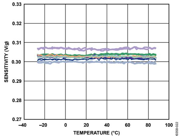
Figure 20. Z-Axis Sensitivity vs. Temperature, Eight Parts Soldered to PCB, V<sub>S</sub> = 3 V
