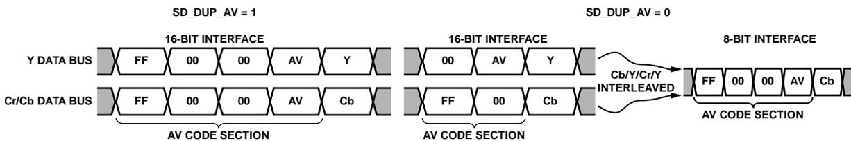
Figure 36. AV Code Duplication Control (64-Lead LQFP Only)
