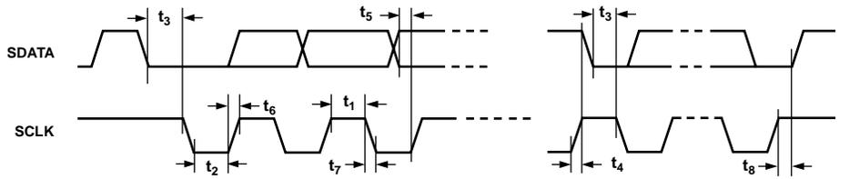
Figure 6. I<sup>2</sup>C Timing
