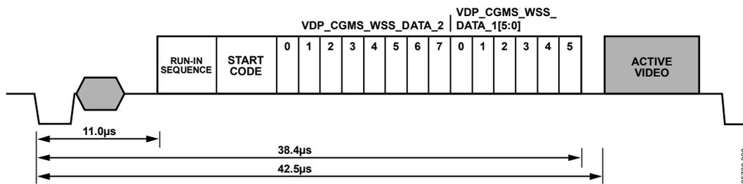
Figure 48. WSS Waveform
