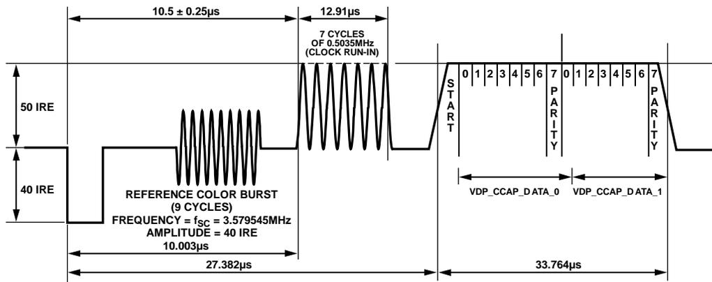
Figure 50. CCAP Waveform and Decoded Data Correlation
