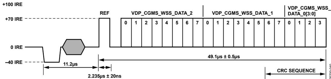
Figure 49. CGMS Waveform
