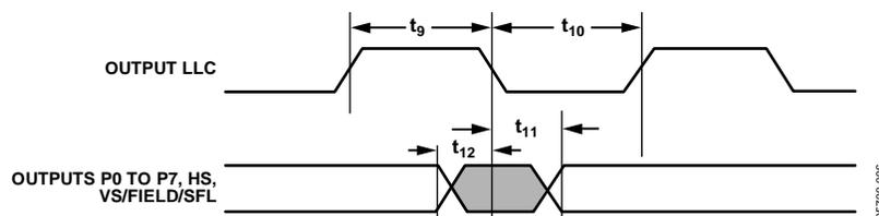
Figure 7. Pixel Port and Control Output Timing
