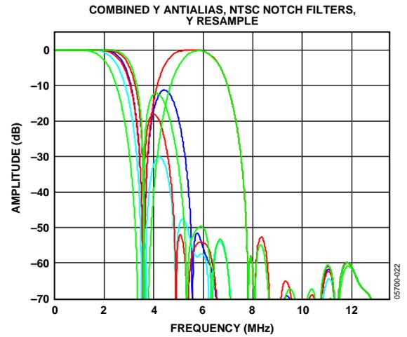
Figure 27. Combined Y Antialias Filter, NTSC Notch Filters
