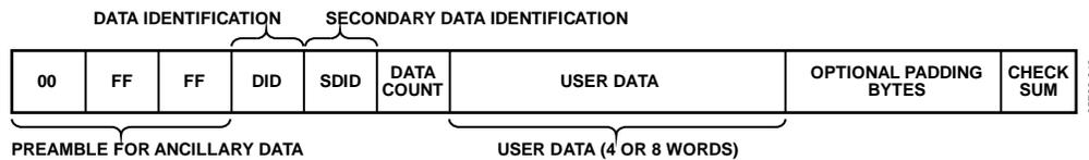
Figure 52. Gemstar- and CCAP-Embedded Data Packet (Generic)
