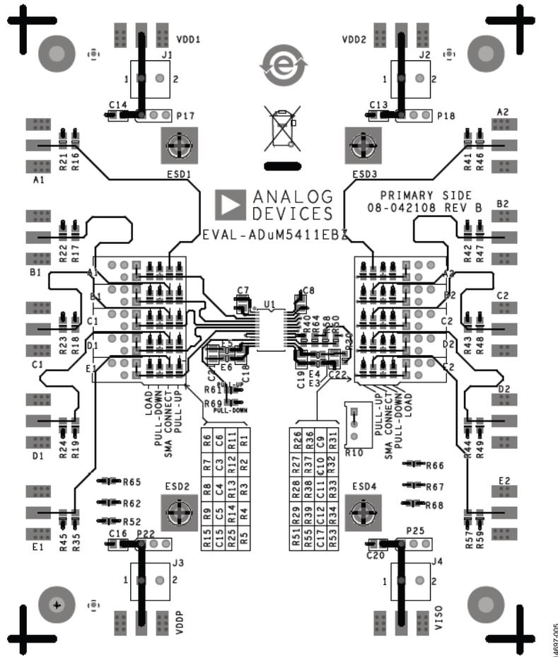
Figure 5. Top Level Signal Routing and Assembly (Layer 1)
