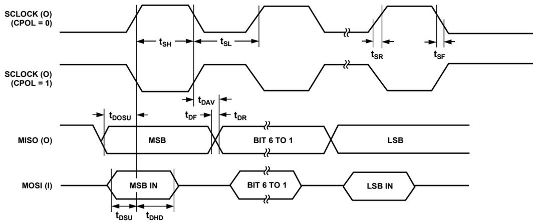
Figure 11. SPI Master Mode Timing (CPHA = 0)
