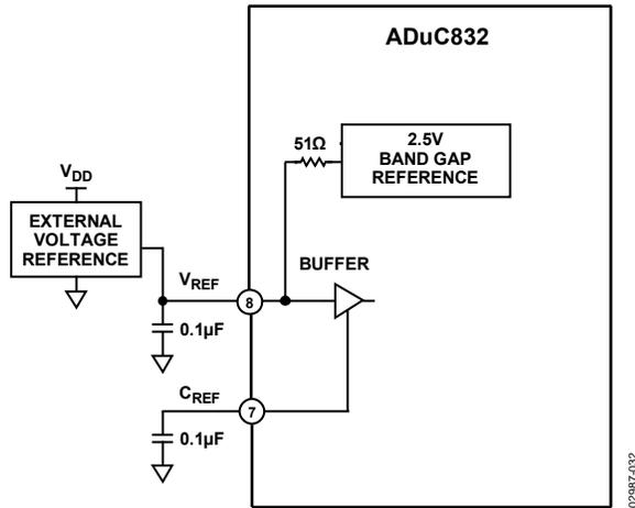
Figure 43. Using an External Voltage Reference
