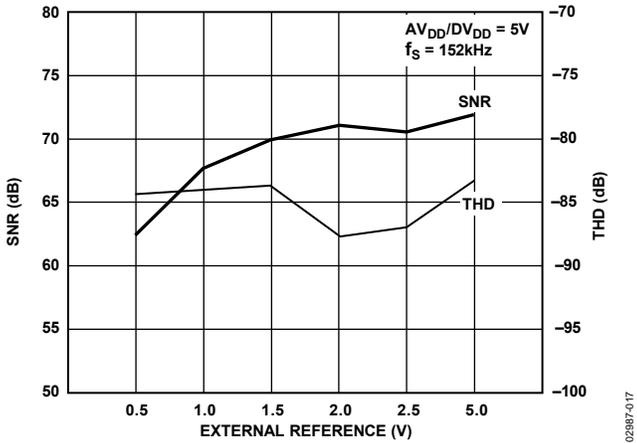
Figure 28. Typical Dynamic Performance vs.  $V_{REF}$ ,  $V_{DD} = 5V$
