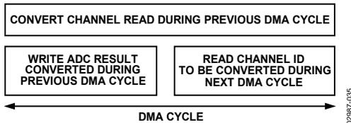
Figure 46. DMA Cycle
