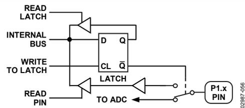
Figure 67. Port 1 Bit Latch and I/O Buffer
