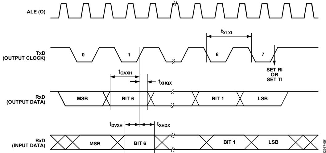
Figure 8. UART Timing in Shift Register Mode
