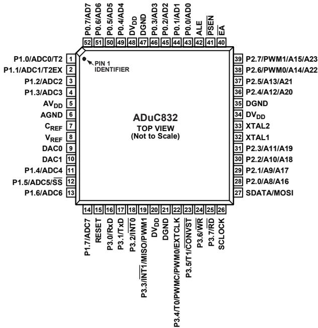
Figure 14. 52-Lead MQFP
