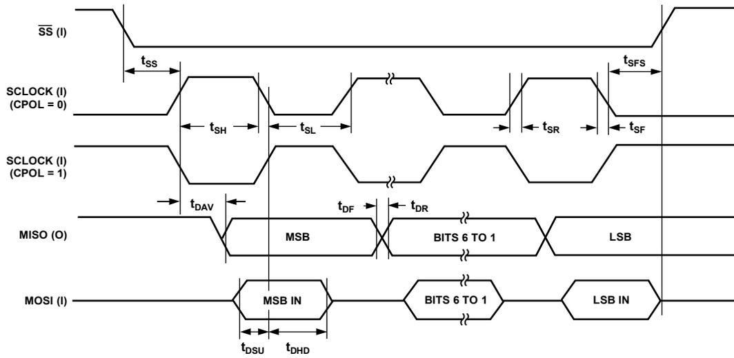
Figure 12. SPI Slave Mode Timing (CPHA = 1)
