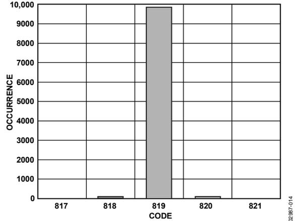
Figure 25. Code Histogram Plot,  $V_{DD} = 3 V$
