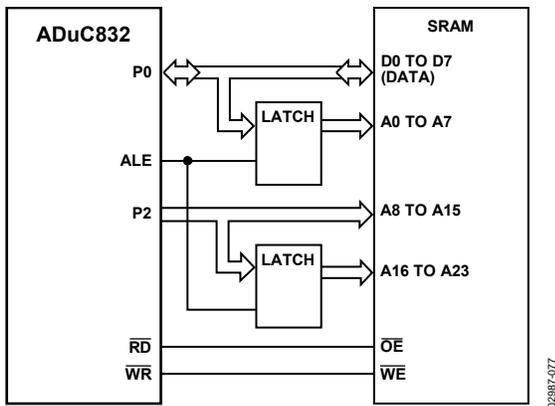
Figure 89. External Data Memory Interface (16 MB Address Space)
