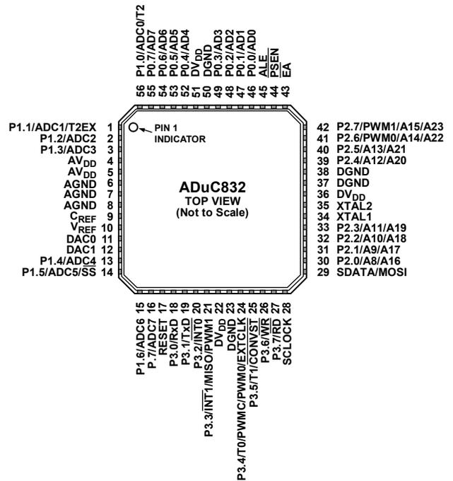
Figure 15. 56-Lead LFCSP
