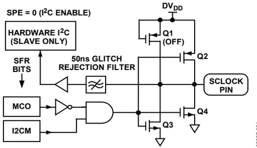
Figure 72. SCLOCK Pin I/O Functional Equivalent in I<sup>2</sup>C Mode
