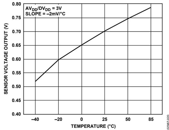
Figure 31. Typical Temperature Sensor Output vs. Temperature
