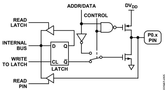
Figure 66. Port 0 Bit Latch and I/O Buffer
