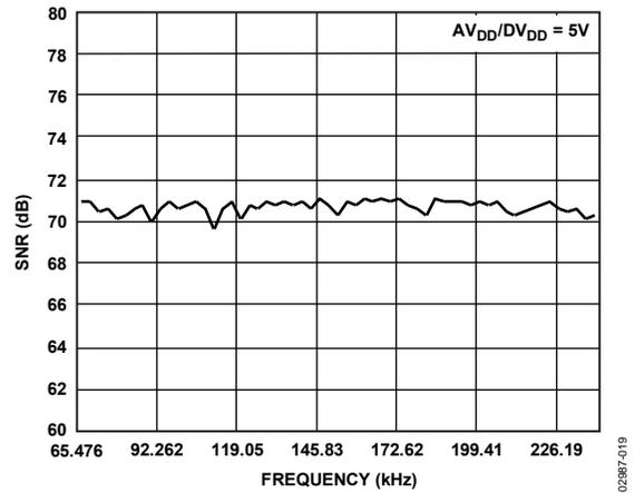
Figure 30. Typical Dynamic Performance vs. Sampling Frequency
