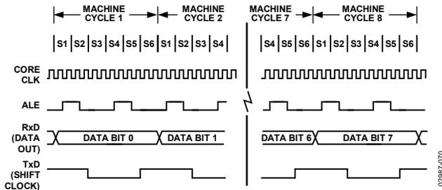
Figure 81. UART Serial Port Transmission, Mode 0
