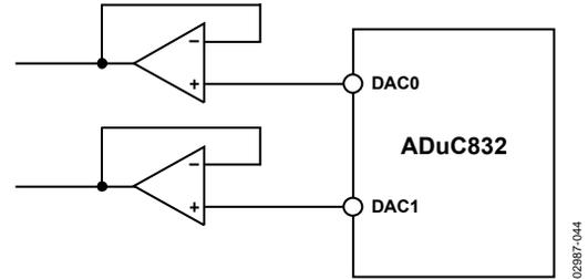
Figure 55. Buffering the DAC Outputs
