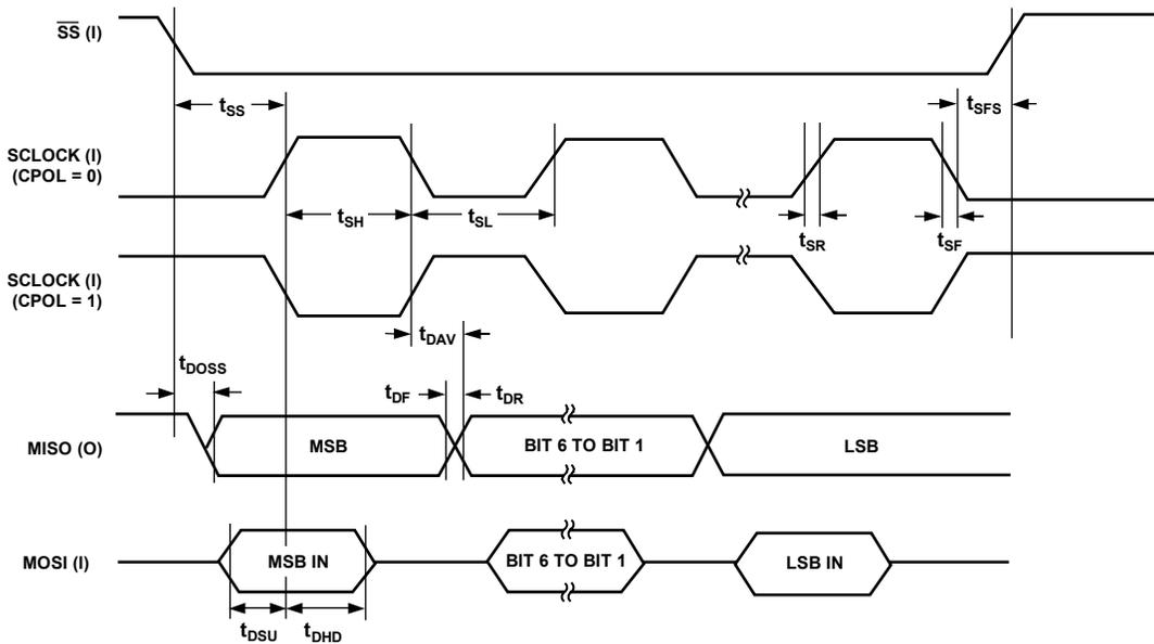
Figure 13. SPI Slave Mode Timing (CPHA = 0)
