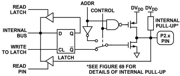
Figure 68. Port 2 Bit Latch and I/O Buffer
