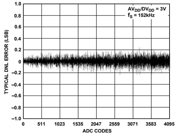
Figure 21. Typical DNL Error,  $V_{DD} = 3V$
