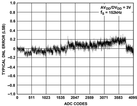
Figure 17. Typical DNL Error,  $V_{DD} = 3V$
