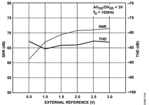
Figure 29. Typical Dynamic Performance vs.  $V_{REF}$ ,  $V_{DD} = 3V$
