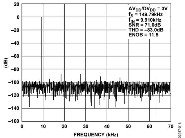
Figure 27. Dynamic Performance at  $V_{DD} = 3 V$
