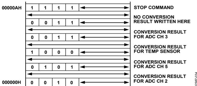
Figure 45. Typical External Memory Configuration Post-ADC DMA Operation
