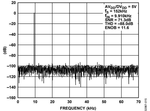
Figure 26. Dynamic Performance at  $V_{DD} = 5 V$
