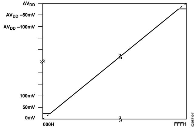
Figure 52. Endpoint Nonlinearities Due to Amplifier Saturation
