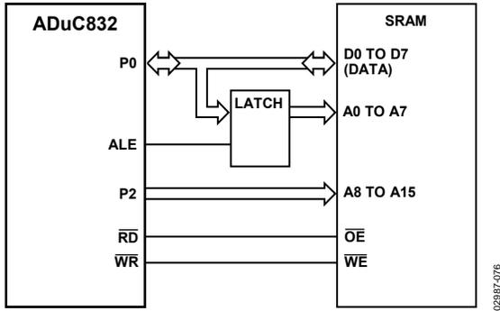
Figure 88. External Data Memory Interface (64 kB Address Space)
