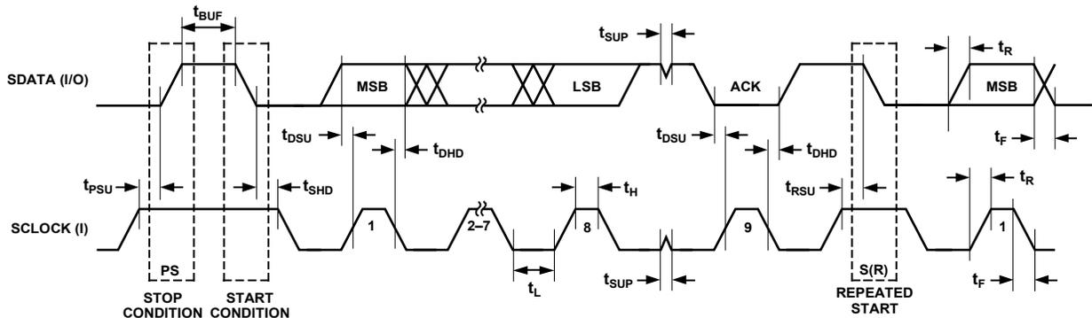
Figure 9. I<sup>2</sup>C Compatible Interface Timing
