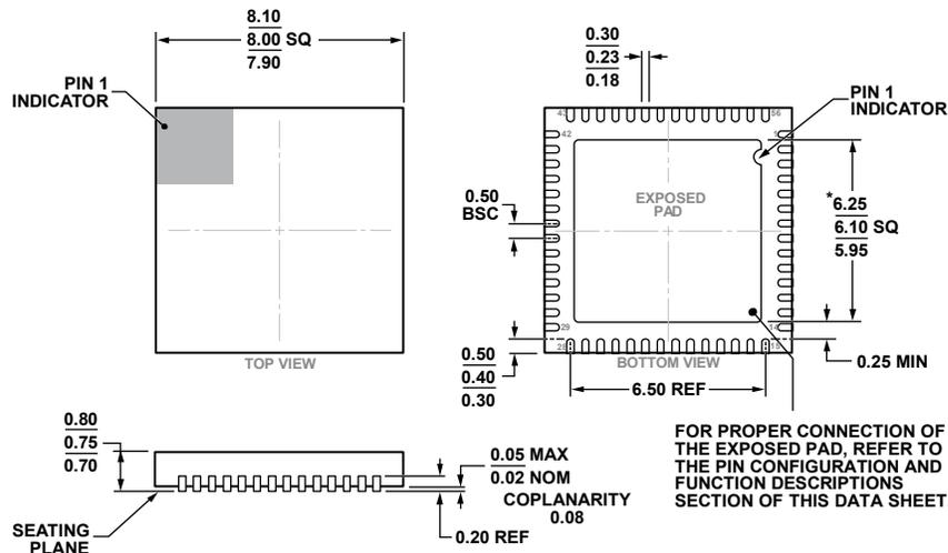
\*COMPLIANT TO JEDEC STANDARDS MO-220-WLLD-2 WITH EXCEPTION TO EXPOSED PAD DIMENSION.
