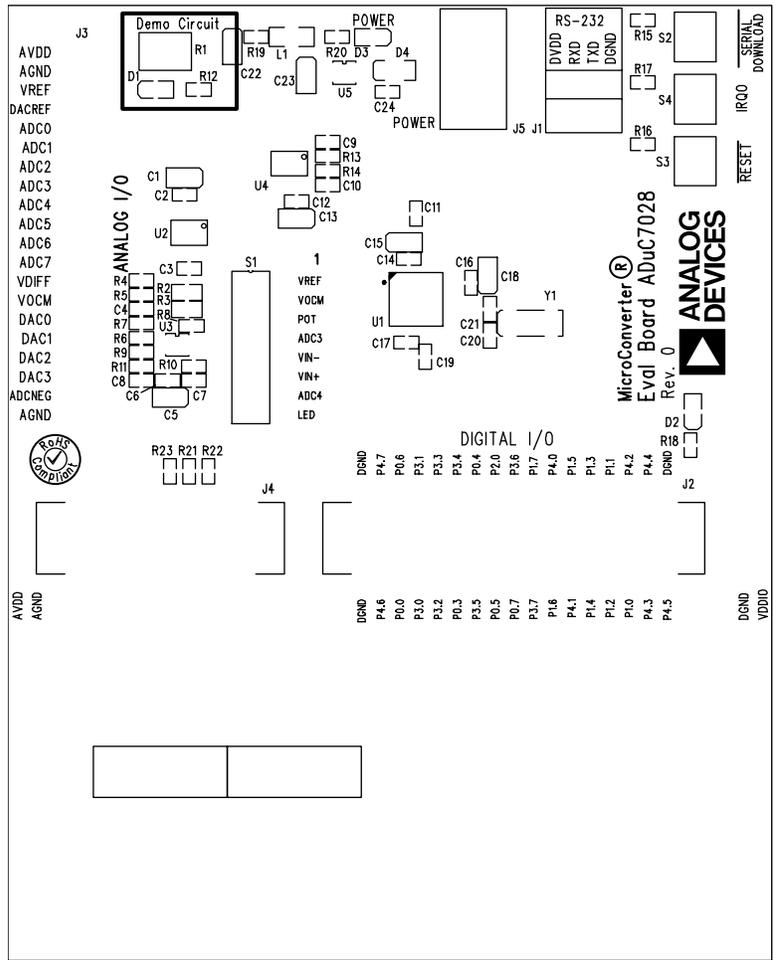
AduC7028 EVALUATION BOARD Rev. 0 – Component Side View
