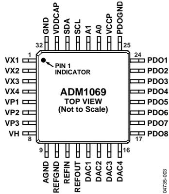
Figure 3. 32-Lead LQFP Pin Configuration
