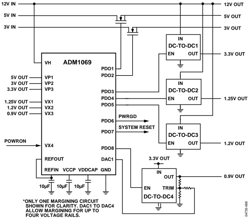
Figure 34. Applications Diagram
