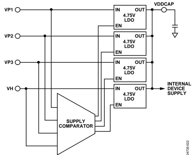
Figure 21. V<sub>DD</sub> Arbitrator Operation
