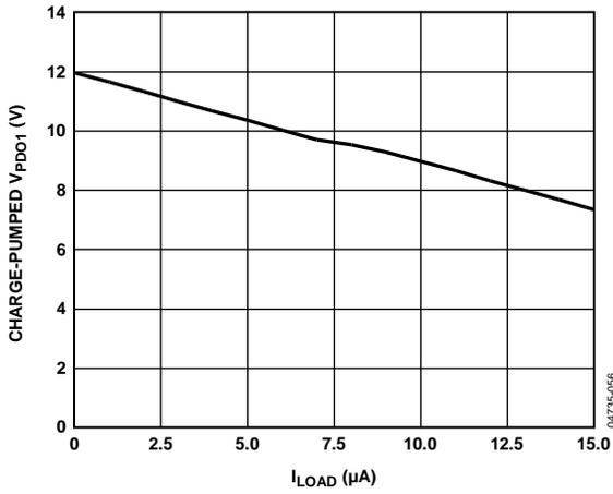
Figure 11. Charge-Pumped  $V_{PDO1}$  (FET Drive Mode) vs.  $I_{LOAD}$
