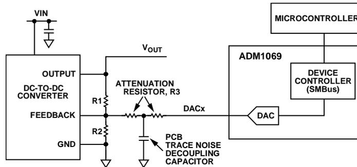
Figure 32. Open-Loop Margining System Using the [ADM1069](#)
