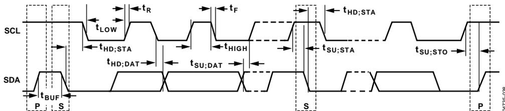
Figure 38. Serial Bus Timing Diagram
