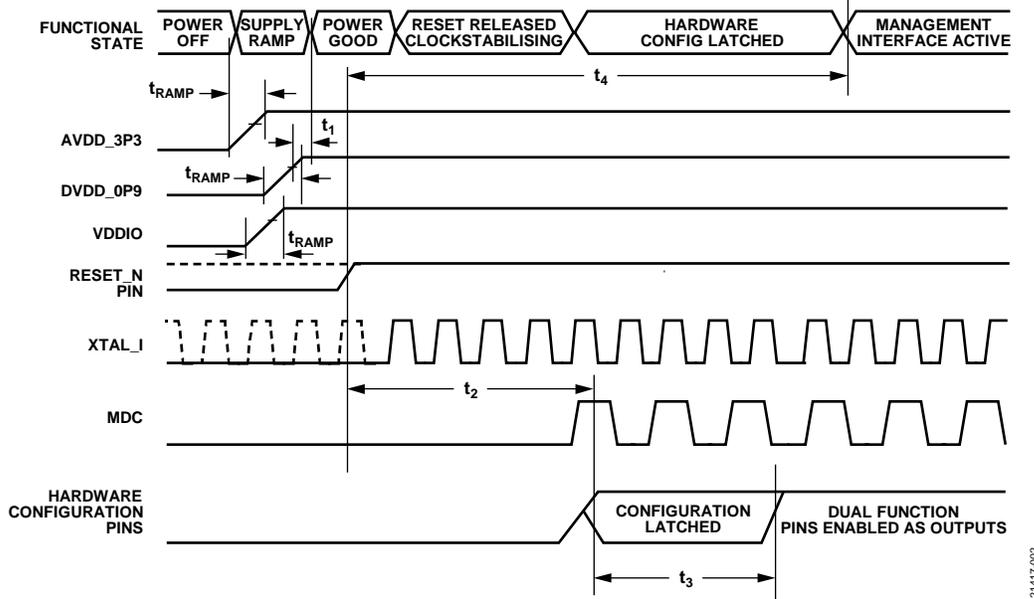
Figure 2. Power-Up Timing
