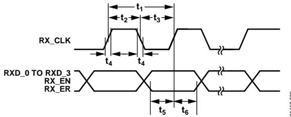
Figure 6. MII Receive Timing
