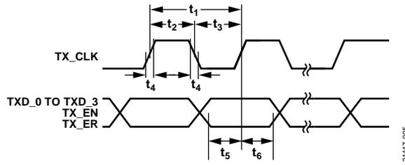
Figure 5. MII Transmit Timing
