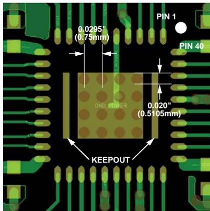
Figure 39. Exposed Paddle Via Array on [EVAL-ADIN1300FMCZ](#)
