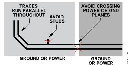
Figure 40. Things to Avoid when Routing Differential Pairs
