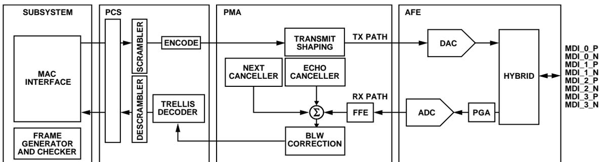
Figure 19. Simplified Channel Block Diagram
