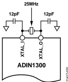
Figure 31. Crystal Oscillator Connection
