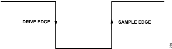
Figure 65. SPI Mode 3, SCLK Edges
