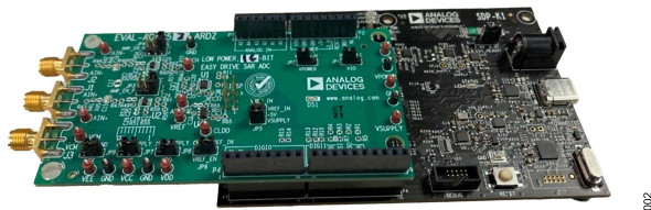
Figure 2. EVAL-AD4052-ARDZ and SDP-K1 Connections
