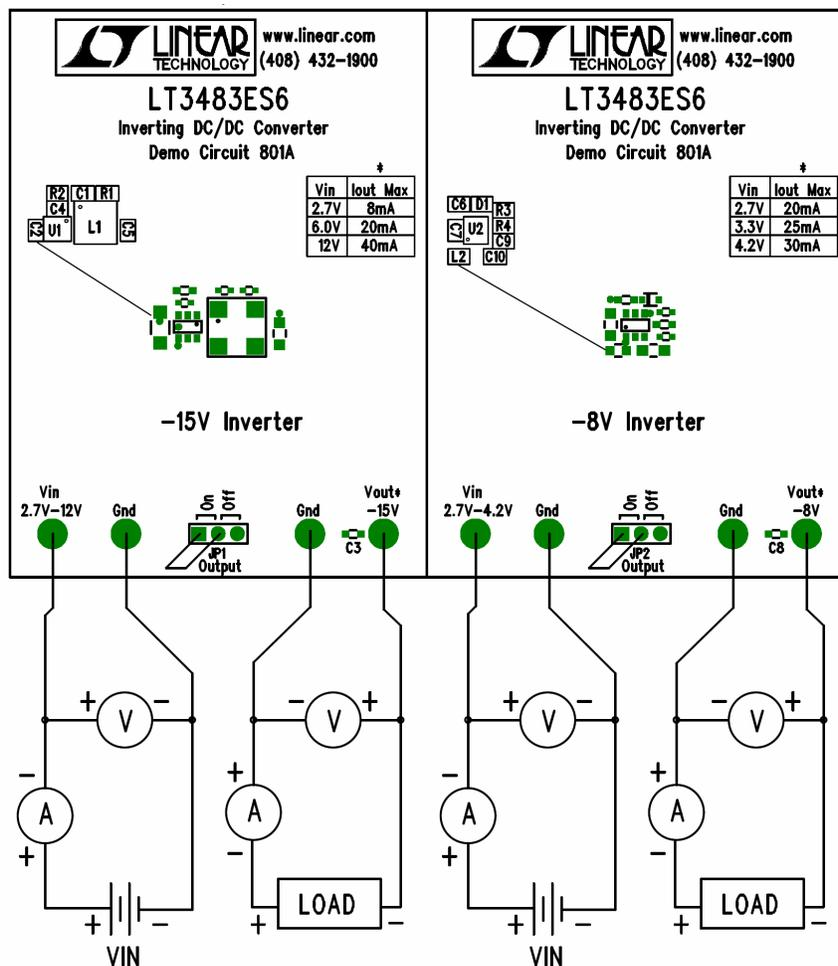
Figure 1. Proper Measurement Equipment Setup
