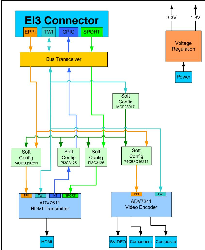
Figure 2-1. Video Encoder EI3 Extender Board Block Diagram
