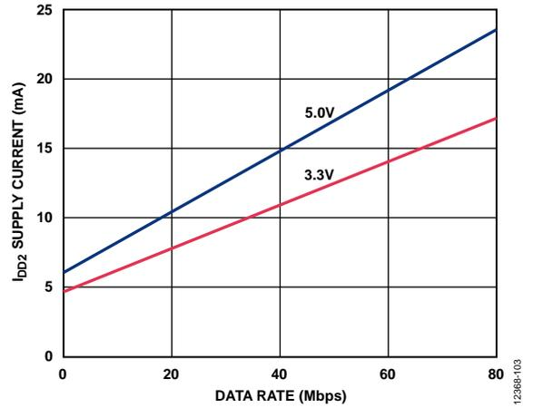
Figure 12. Typical I<sub>DD2</sub> Supply Current vs. Data Rate for 5.0 V and 3.3 V Operation
