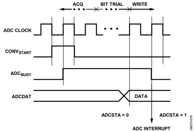
Figure 23. ADC Timing
