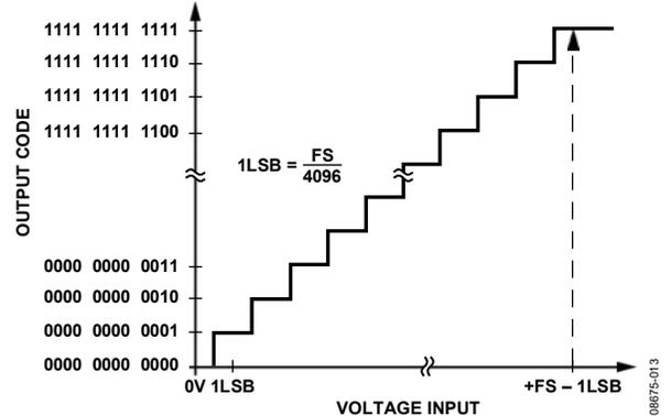
Figure 20. ADC Transfer Function in Single-Ended Mode
