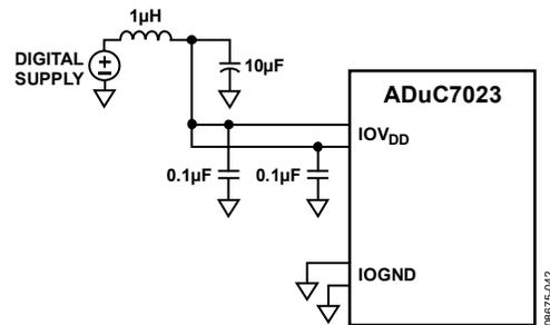
Figure 48. Recommended IOV<sub>DD</sub> Supply Filter
