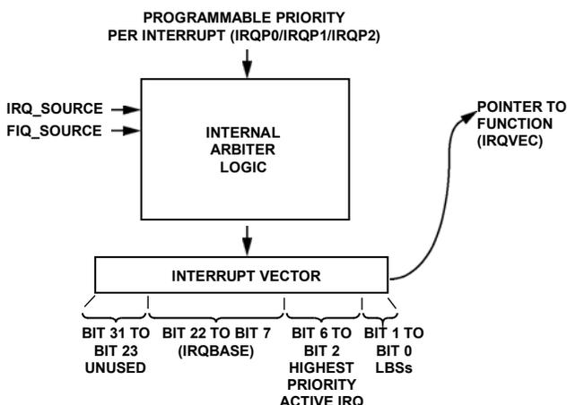
Figure 41. Interrupt Structure
