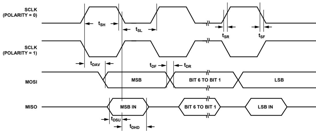
Figure 3. SPI Master Mode Timing (Phase Mode = 1)
