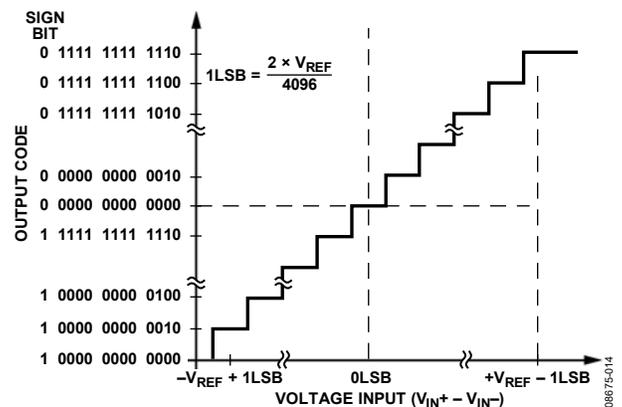
Figure 21. ADC Transfer Function in Differential Mode
