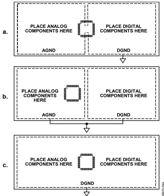
Figure 50. System Grounding Schemes
