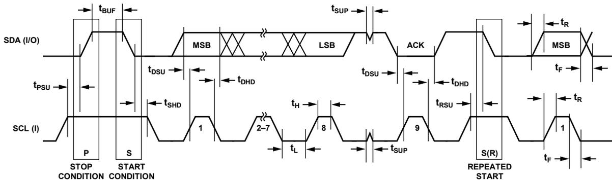
Figure 2. I<sup>2</sup>C-Compatible Interface Timing
