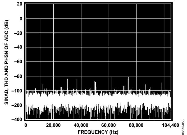
Figure 14. SINAD, THD, and PHSN of ADC, Internal 2.5 V Reference Used
