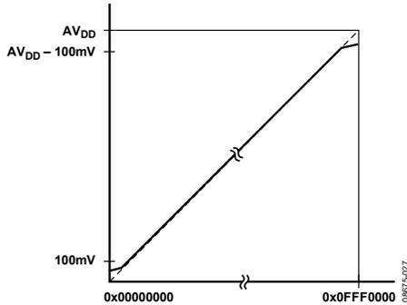
Figure 33. Endpoint Nonlinearities Due to Amplifier Saturation
