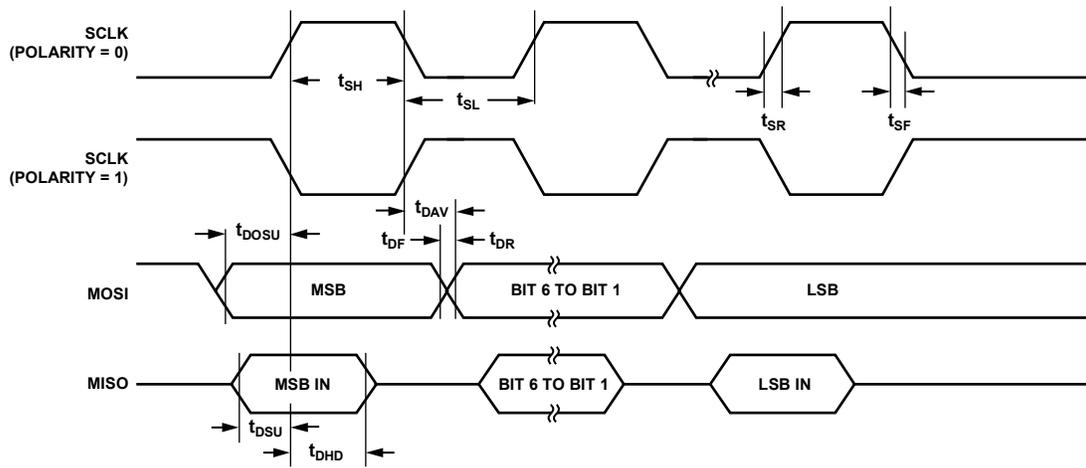
Figure 4. SPI Master Mode Timing (Phase Mode = 0)
