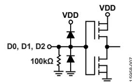
Figure 7. Digital Input Interface (D0, D1, D2)
