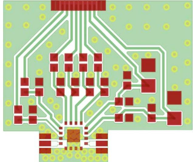
Figure 32. Probe Matrix Board Layout (Top View)
