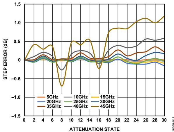
Figure 13. Step Error vs. Attenuation State over Frequency
