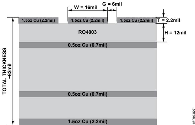
Figure 27. Evaluation Board Stackup, Cross Sectional View
