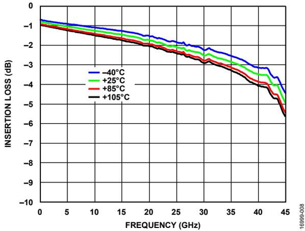
Figure 8. Insertion Loss vs. Frequency over Temperature
