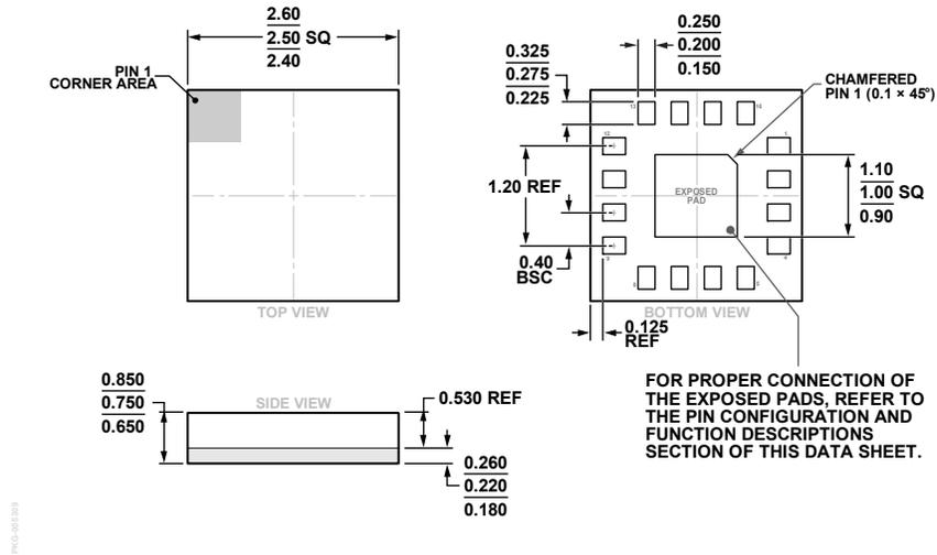
Figure 34. 16-Terminal Land Grid Array [LGA]
