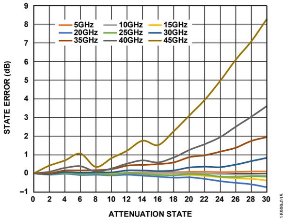
Figure 15. State Error vs. Attenuation State over Frequency
