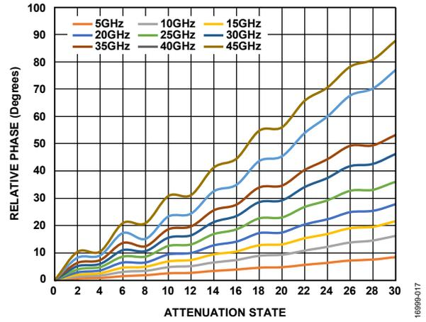
Figure 17. Relative Phase vs. Attenuation State over Frequency
