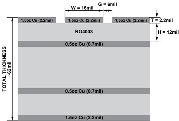
Figure 31. Probe Matrix Board (Cross Sectional View)
