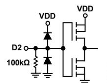
Figure 7. Digital Input Interface Schematic for D2
