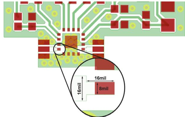
Figure 33. Probe Board Layout Dimensions (Top View)
