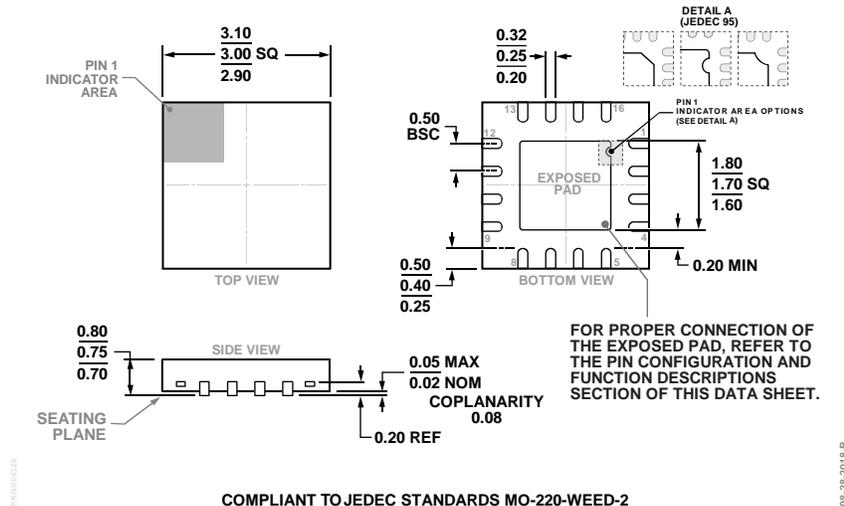
Figure 18. 16-Lead Lead Frame Chip Scale Package [LFCSP]
