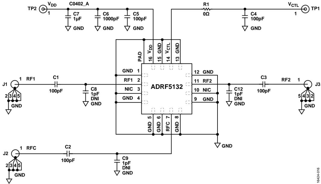
Figure 17. Application Circuit
