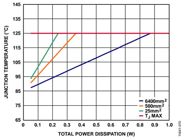
Figure 76. SOIC, T<sub>A</sub> = 85°C
