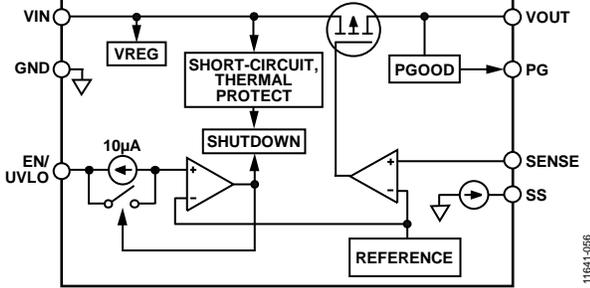
Figure 60. Fixed Output Voltage Internal Block Diagram
