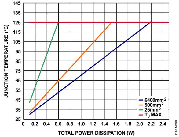
Figure 74. SOIC, T<sub>A</sub> = 25°C
