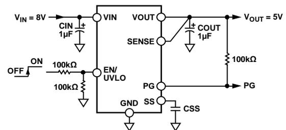
Figure 1. **ADP7105** with Fixed Output Voltage, 5 V
