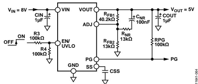
Figure 70. Noise Reduction Modification to Adjustable LDO Regulator
