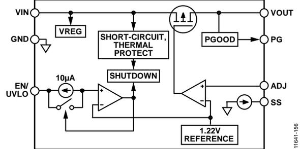
Figure 61. Adjustable Output Voltage Internal Block Diagram
