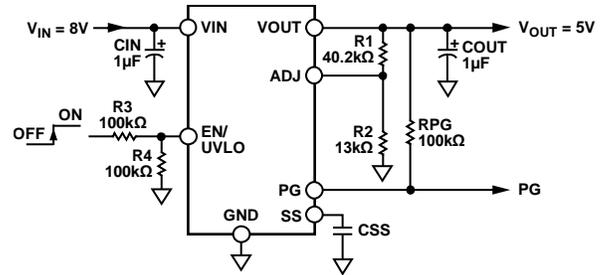
Figure 62. Typical Adjustable Output Voltage Application Schematic
