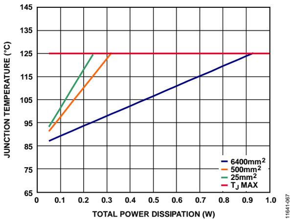
Figure 73. LFCSP, T<sub>A</sub> = 85°C
