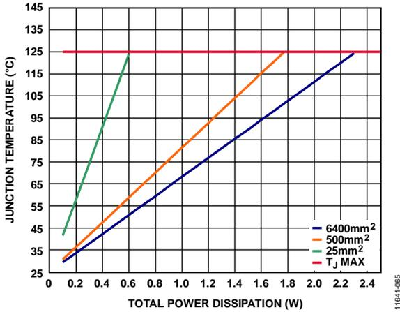
Figure 71. LFCSP, T<sub>A</sub> = 25°C
