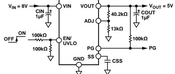
Figure 2. **ADP7105** with Adjustable Output Voltage, 5 V
