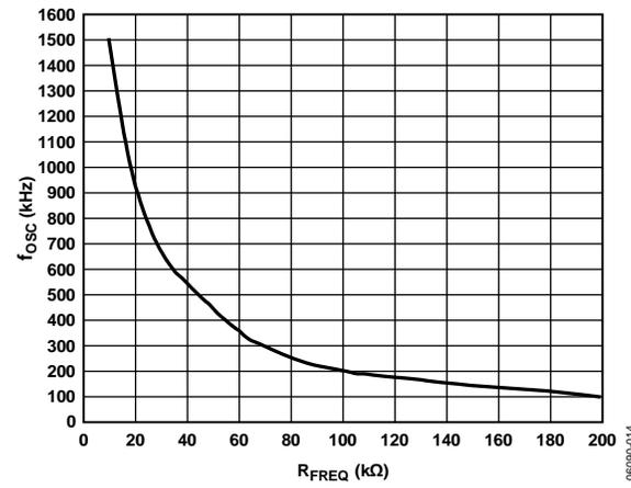
Figure 15. Oscillator Frequency vs. Resistance
