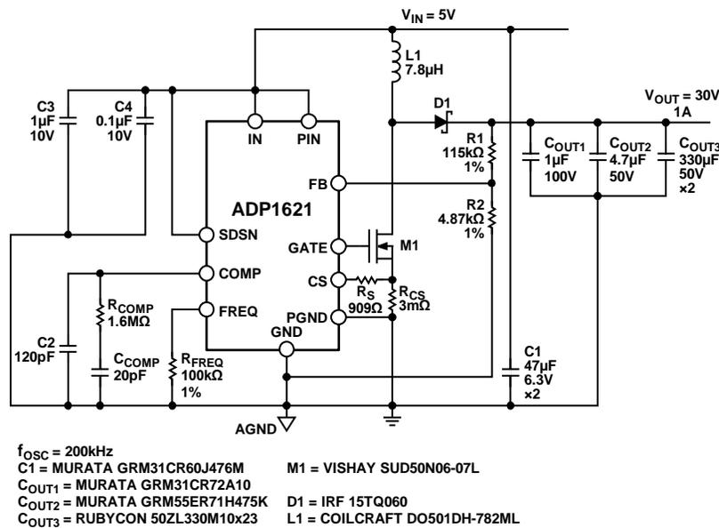
Figure 36. Low Input, High Output Boost Converter
