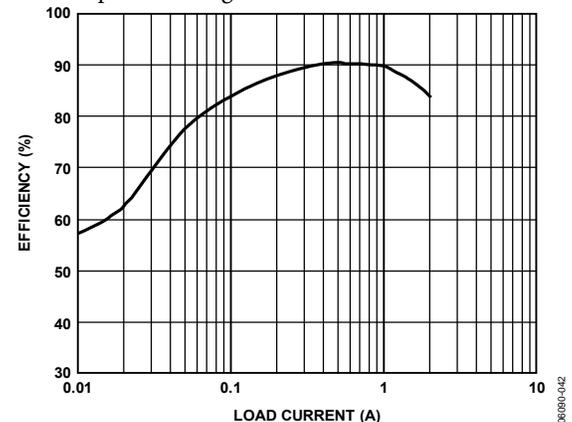
Figure 2. Efficiency of Circuit Shown in Figure 1
