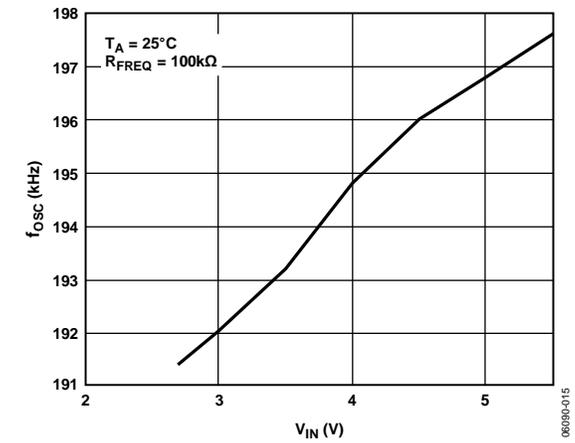
Figure 16. Oscillator Frequency vs.  $V_{IN}$
