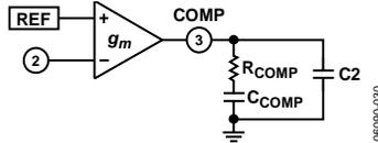
Figure 31. Compensation Components
