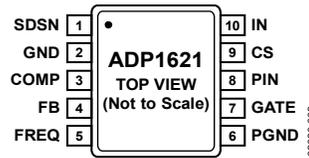
Figure 4. Pin Configuration
