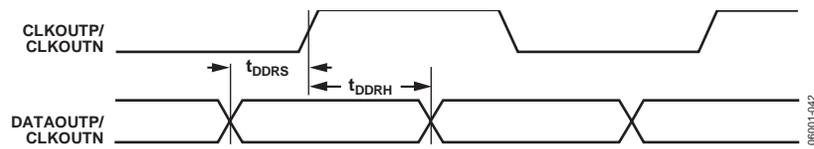
Figure 4. Double Data Rate Mode Output Timing
