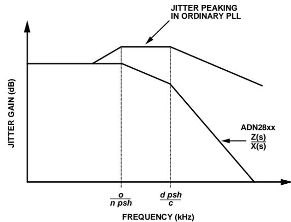
Figure 29. ADN2817/ADN2818 Jitter Response vs. Conventional PLL
