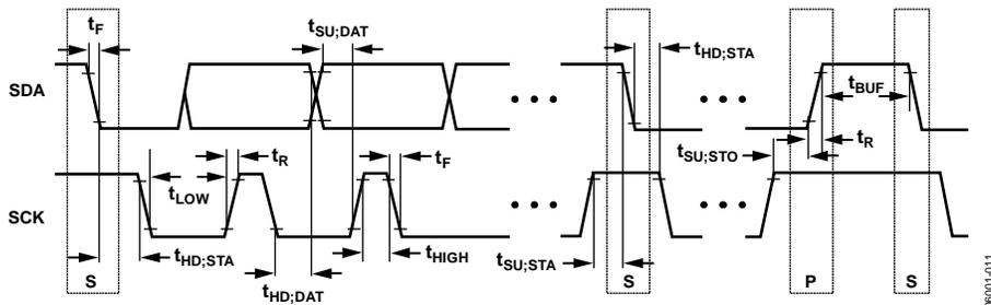
Figure 22. I<sup>2</sup>C Port Timing Diagram
