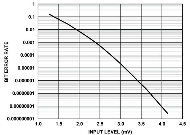
Figure 17. Bit Error Rate vs. Input Level
