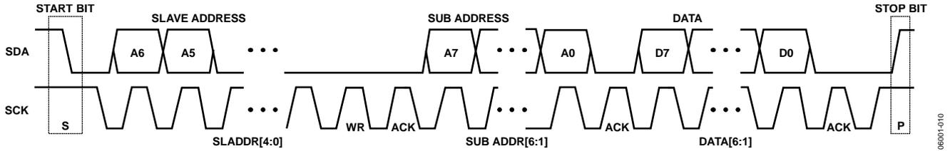
Figure 21. I<sup>2</sup>C Data Transfer Timing
