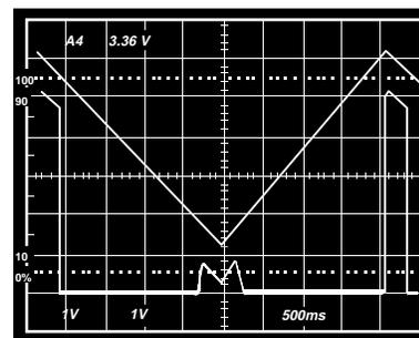
Figure 1. RESET Output Voltage vs. V<sub>CC</sub>
