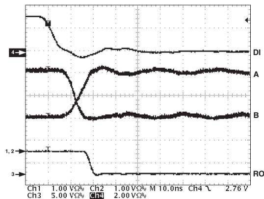
TPC 16. Driver/Receiver Propagation Delays High to Low
