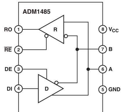
This minimizes the loading effect when the transceiver is not being used. The high impedance driver output is maintained over the entire common-mode voltage range from -7 V to +12 V.
