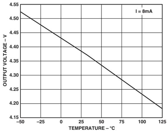
TPC 3. Receiver Output High Voltage vs. Temperature
