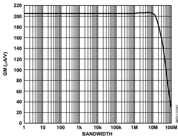
Figure 12.  $C_{CMP}$  and  $S_{CMP}$  Transconductance
