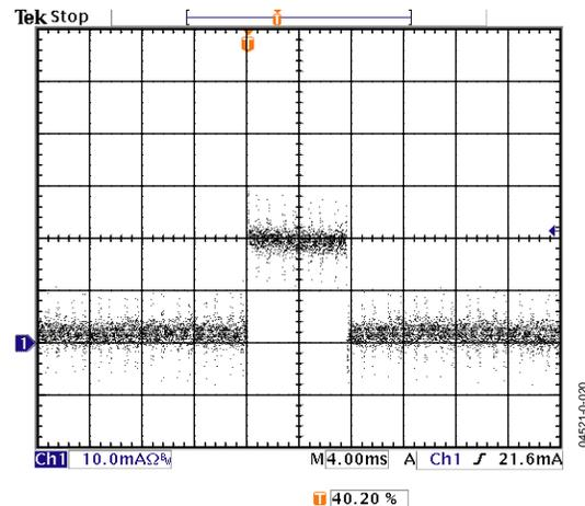
Figure 29. EEPROM Page Erase Peak  $I_{DD}$  Current
