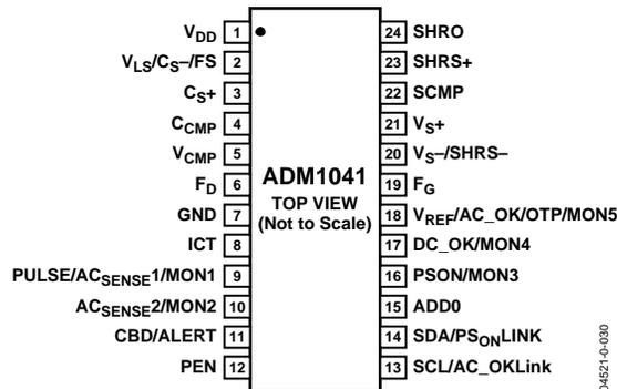
Figure 7. Pin Configuration
