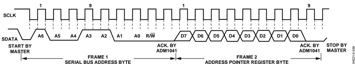
Figure 26. Writing to the Address Pointer Register Only
