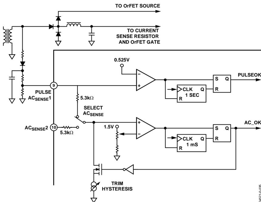
Figure 16. Pulse In and AC Sense Circuit
