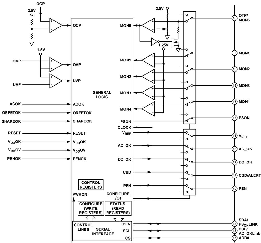
Figure 23. Block Diagram of Protection and General Logic
