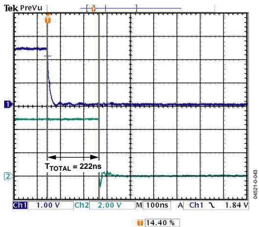
Figure 19. OrFET Turn- Off Time (Inverse Polarity)
