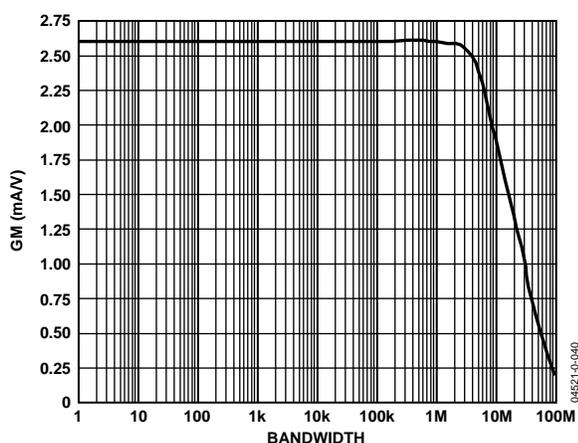
Figure 11.  $V_{CMP}$  Transconductance
