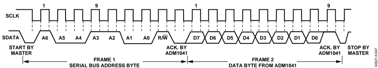
Figure 27. Reading Data from a Previously Selected Register
