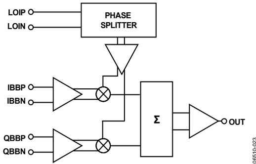
Figure 22. Block Diagram
