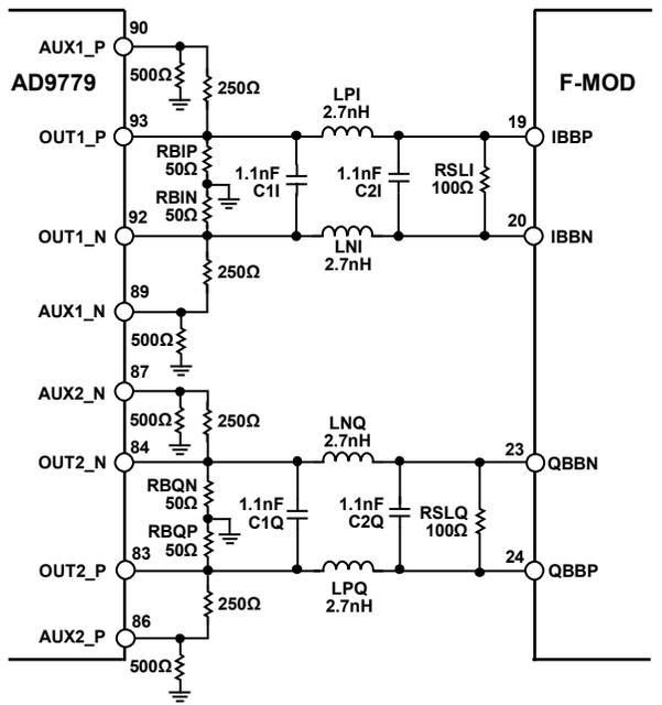
Figure 31. DAC Modulator Interface with Auxiliary DAC Resistors
