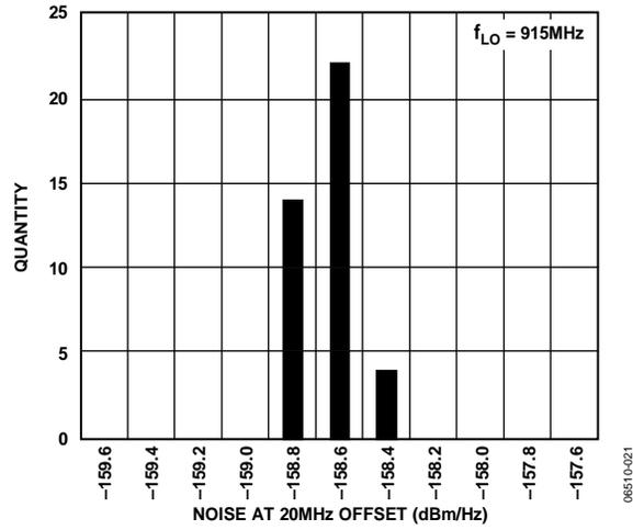
Figure 21. 20 MHz Offset Noise Floor Distribution at  $f_{LO} = 915\text{MHz}$
