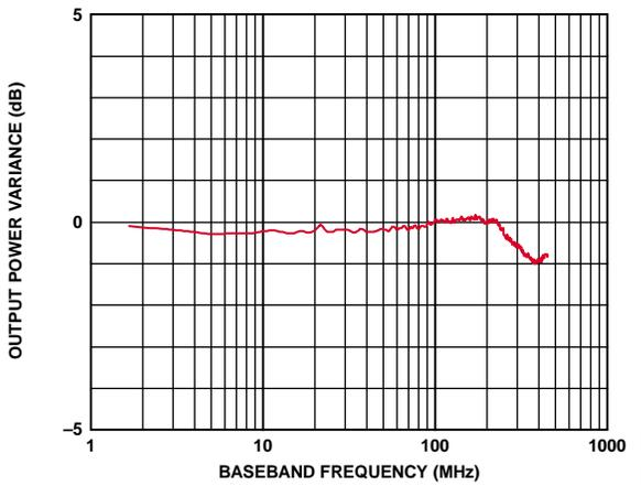
Figure 5. I/Q Input Bandwidth Normalized to Gain @ 1 MHz ( $f_{LO} = 900$  MHz)
