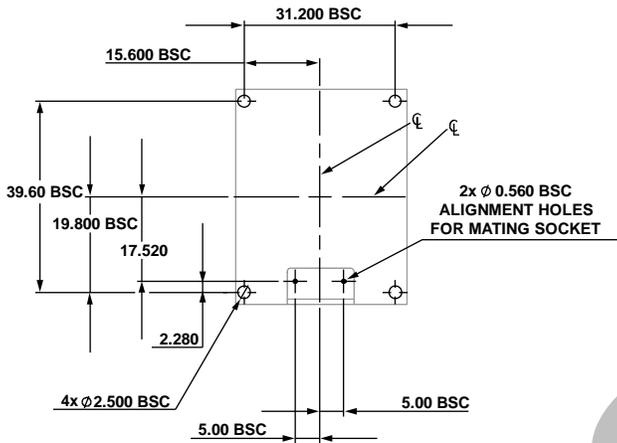
Figure 23. Suggested Mounting Hole Locations, Connector Down
