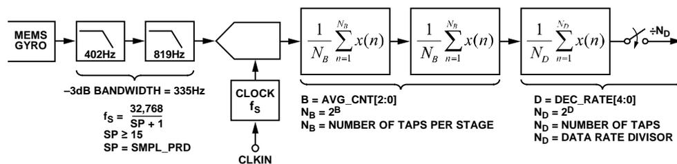
Figure 18. Sampling and Frequency Response Block Diagram
