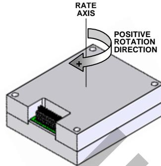
Figure 6. Axial Orientation (Bottom Side Facing Up)
