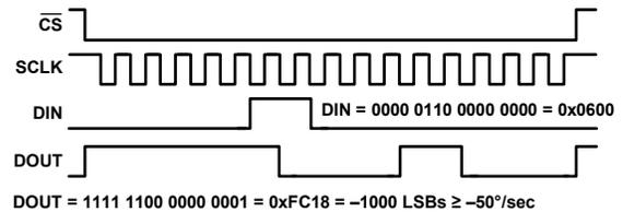
Figure 12. SPI Read Example, Second 16-Bit Sequence
