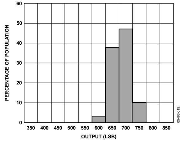
Figure 16. Self-Test at 25°C, V<sub>CC</sub> at 5.0 V
