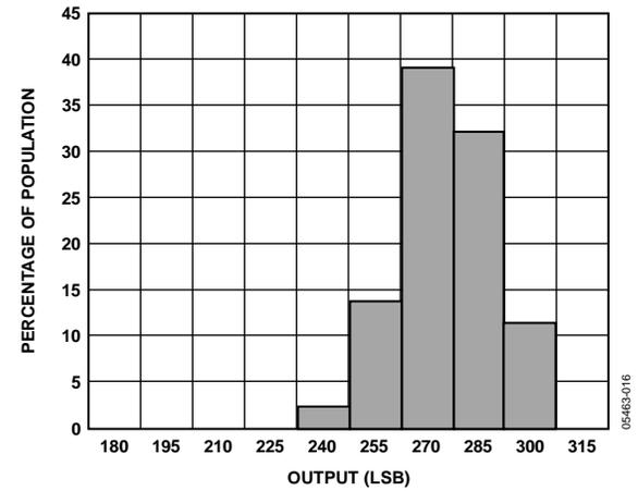
Figure 17. Self-Test at 25°C, V<sub>CC</sub> at 3.3 V
