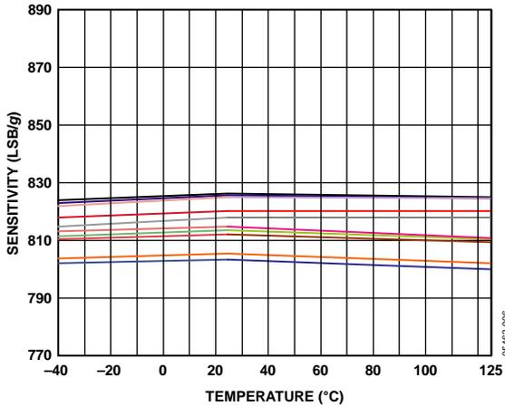
Figure 7. Sensitivity vs. Temperature (ADIS16003 Soldered to PCB)
