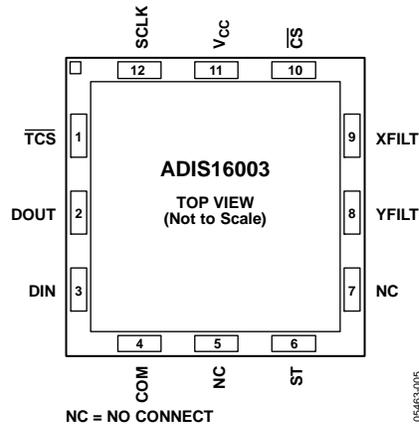
Figure 6. Pin Configuration
