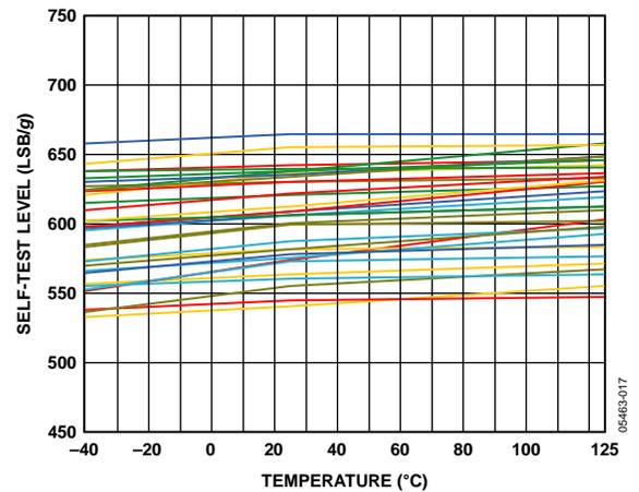
Figure 18. Self-Test vs. Temperature, V<sub>CC</sub> at 5.0 V
