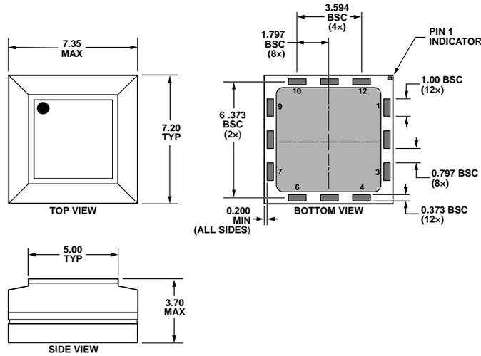
Figure 24. 12-Terminal Land Grid Array [LGA]
