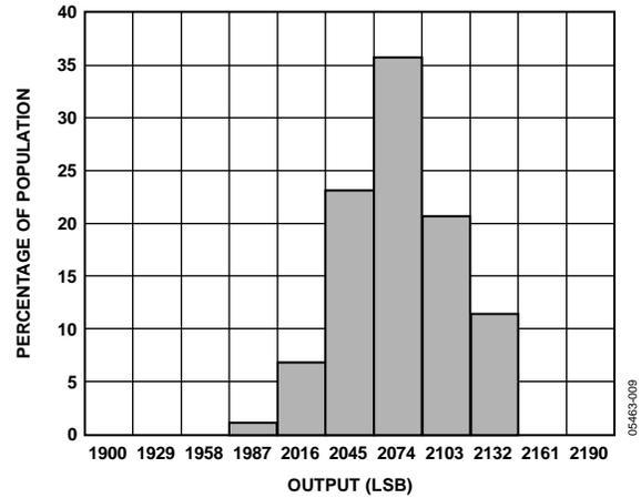
Figure 10. X-Axis Zero g Bias at 25°C
