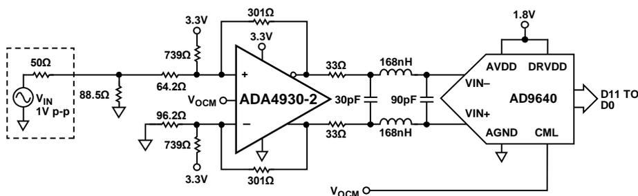
Figure 60. Driving an AD9640, 14-Bit, 80 MSPS ADC
