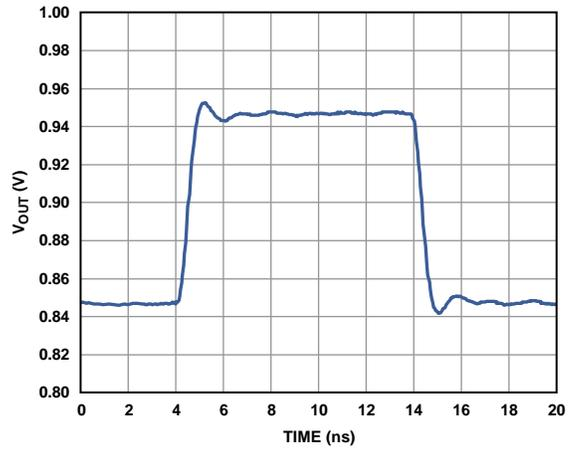
Figure 35. Small Signal  $V_{OCM}$  Pulse Response
