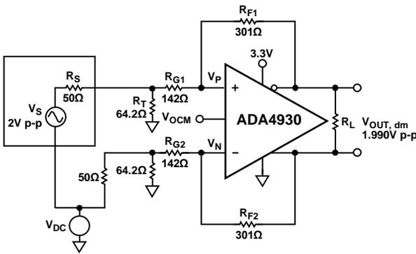
Figure 51. Single-Supply, Terminated Single-Ended-to-Differential System with  $G = 1$
