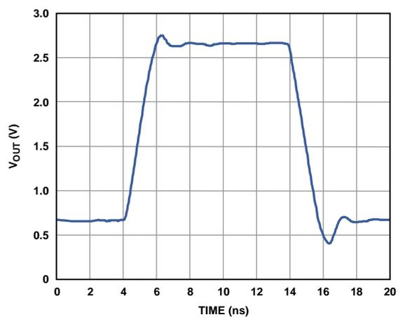
Figure 36. Large Signal  $V_{OCM}$  Pulse Response
