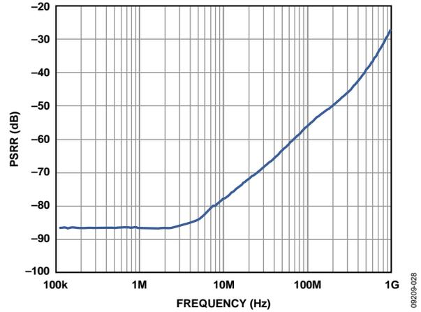
Figure 28. PSRR vs. Frequency,  $R_L = 200 \Omega$
