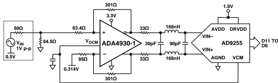
Figure 59. Driving an AD9255, 14-Bit, 80 MSPS ADC
