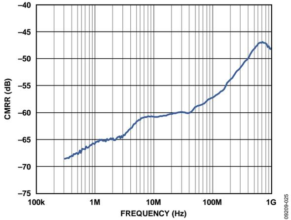
Figure 25. CMRR vs. Frequency,  $R_L = 200 \Omega$
