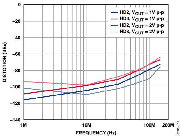
Figure 21. Distortion vs.  $V_{OUT}$  at  $V_S = 3.3V$
