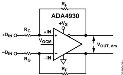
Figure 44. ADA4930-1/ADA4930-2 Configured for Balanced (Differential) Inputs
