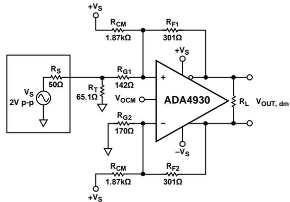
Figure 55. Single-Supply, Single-Ended Input System with Bias Resistors
