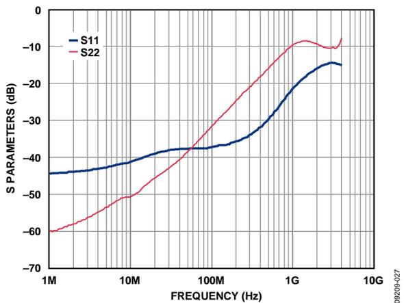
Figure 27.  $S_{11}$ ,  $S_{22}$ ,  $R_L = 200 \Omega$
