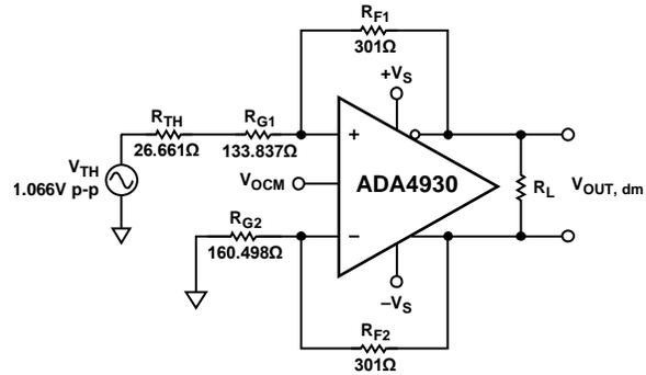
Figure 49. Thevenin Equivalent with Matched Gain Resistors
