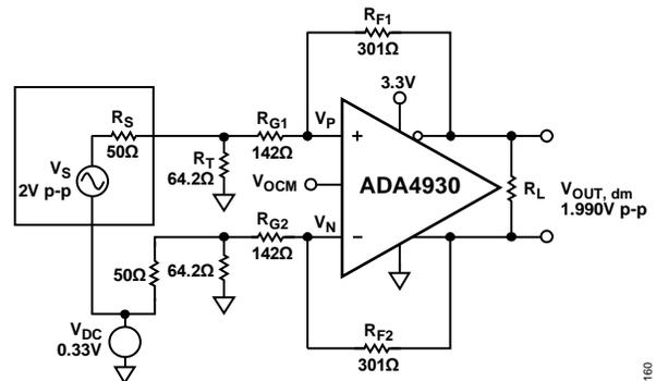
Figure 53. Single-Supply Application Circuit with DC Source Bias
