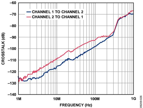
Figure 26. Crosstalk vs. Frequency,  $R_L = 200 \Omega$
