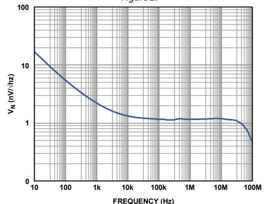
Figure 3. Voltage Noise Spectral Density
