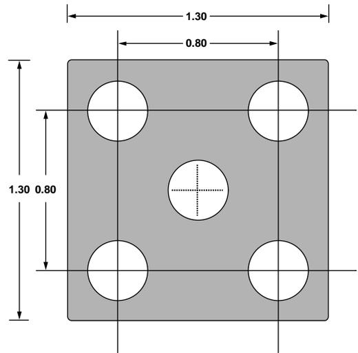
Figure 57. Recommended PCB Thermal Attach Pad Dimensions (Millimeters)
