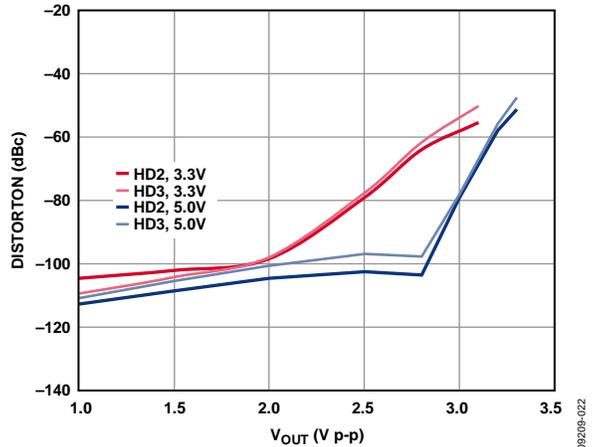
Figure 22. Harmonic Distortion vs. Output @ 10MHz
