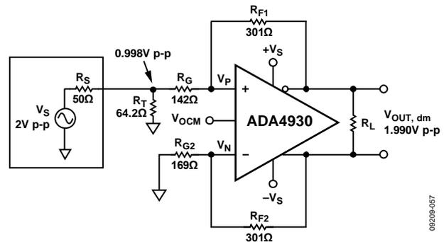
Figure 50. Terminated Single-Ended-to-Differential System with  $G = 1$
