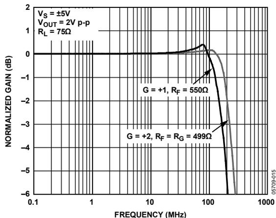
Figure 12. Large Signal Frequency Response for Various Gains
