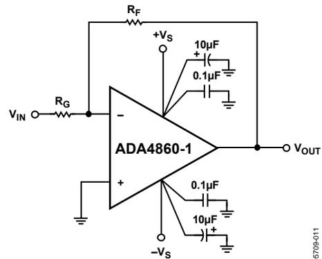
Figure 52. Inverting Gain
