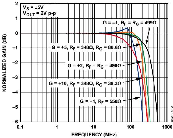
Figure 5. Large Signal Frequency Response for Various Gains
