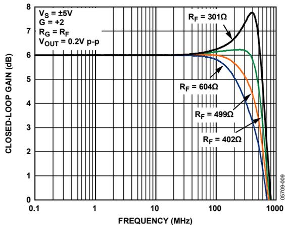
Figure 10. Small Signal Frequency Response vs.  $R_f$
