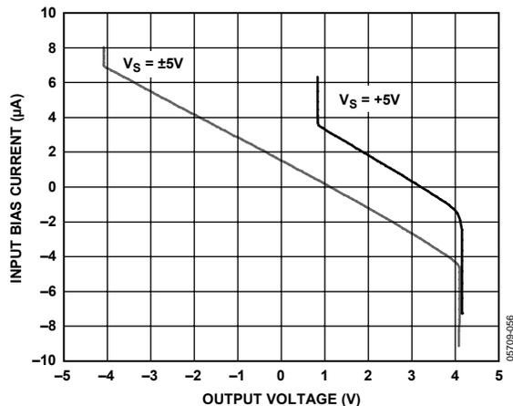
Figure 48. Inverting Input Bias Current vs. Output Voltage
