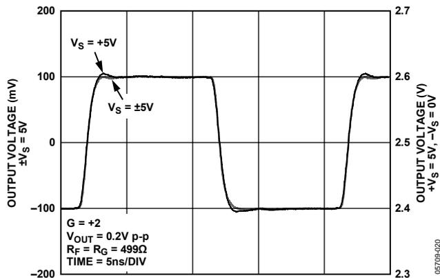
Figure 25. Small Signal Transient Response for Various Supplies
