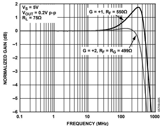
Figure 14. Small Signal Frequency Response for Various Gains
