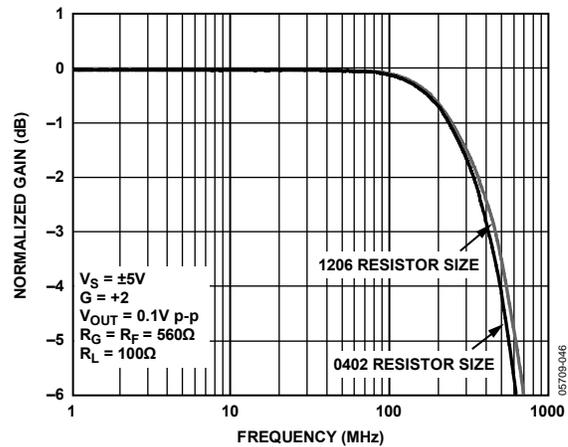
Figure 59. Small Signal Frequency Response vs. Resistor Size
