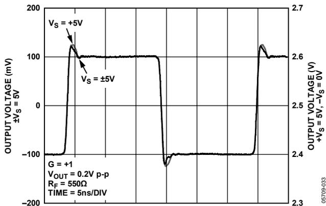
Figure 22. Small Signal Transient Response for Various Supplies
