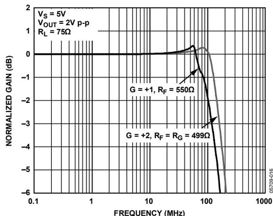
Figure 15. Large Signal Frequency Response for Various Gains
