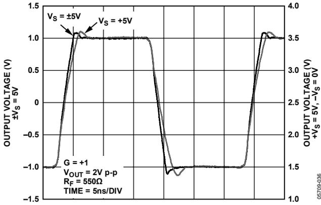
Figure 28. Large Signal Transient Response for Various Supplies
