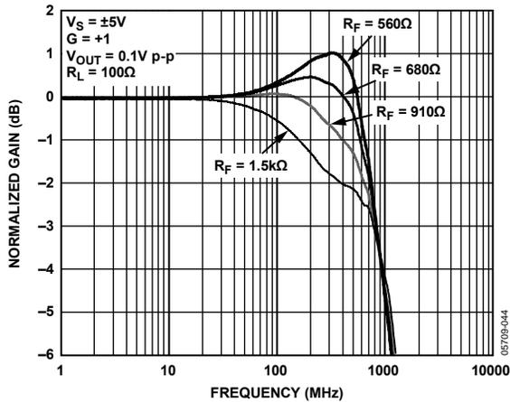
Figure 56. Small Signal Frequency Response vs.  $R_f$
