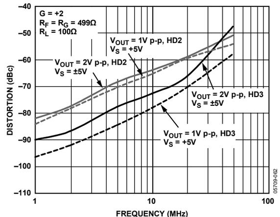
Figure 21. Harmonic Distortion vs. Frequency for Various Supplies
