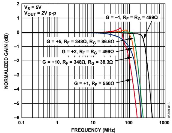
Figure 8. Large Signal Frequency Response for Various Gains
