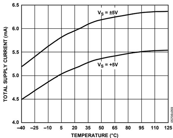
Figure 47. Supply Current at Various Supplies vs. Temperature
