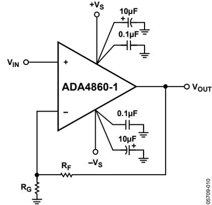
Figure 51. Noninverting Gain
