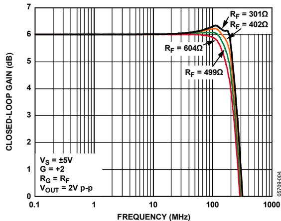
Figure 13. Large Signal Frequency Response vs.  $R_f$
