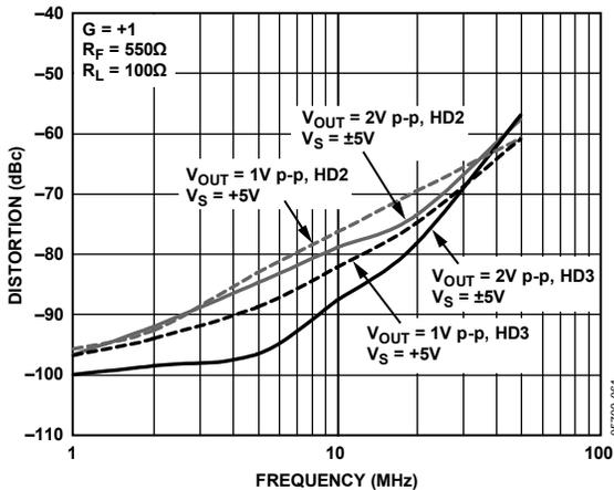
Figure 18. Harmonic Distortion vs. Frequency for Various Supplies
