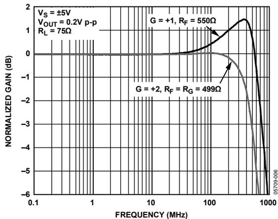
Figure 11. Small Signal Frequency Response for Various Gains
