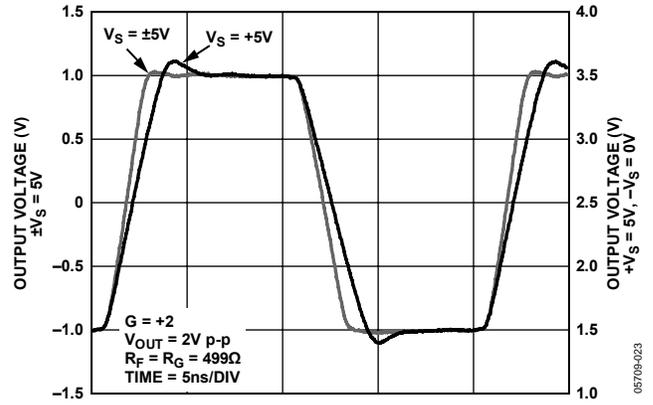
Figure 31. Large Signal Transient Response for Various Supplies
