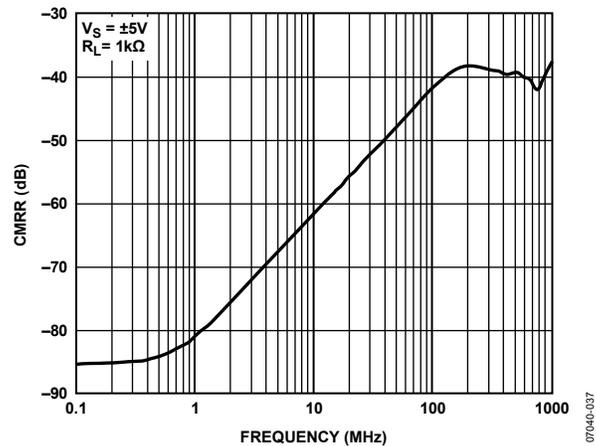
Figure 37. Common-Mode Rejection Ratio (CMRR) vs. Frequency
