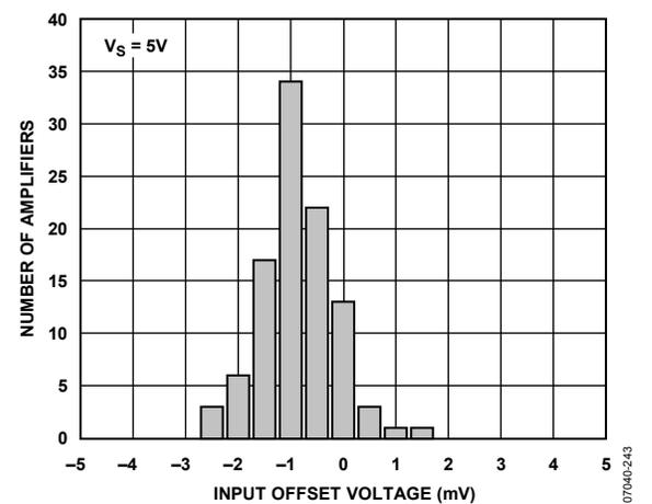
Figure 43. Input Offset Voltage Distribution,  $V_S = 5 V$
