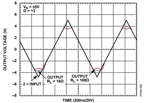
Figure 36. Output Overdrive Recovery for Various Resistive Loads
