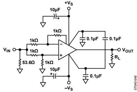
Figure 52. Common-Mode Rejection
