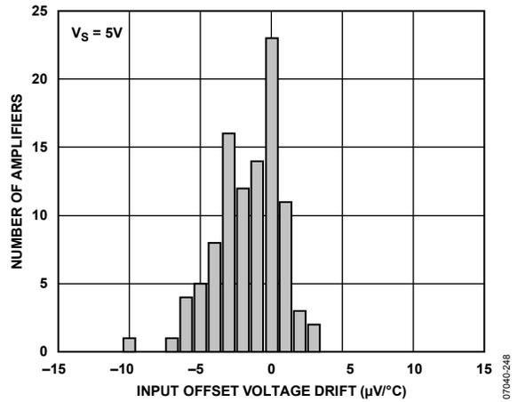
Figure 48. Input Offset Voltage Drift Distribution,  $V_S = 5V$
