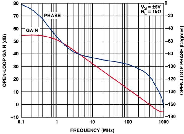
Figure 32. Open-Loop Gain and Phase vs. Frequency
