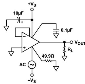
Figure 53. Negative Power Supply Rejection
