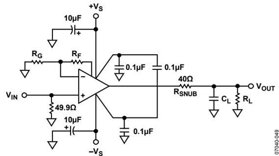
Figure 54. Typical Capacitive Load Configuration (SOIC)
