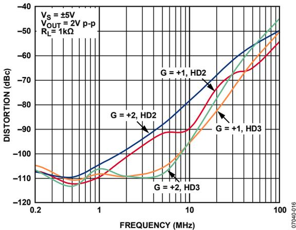
Figure 16. Harmonic Distortion vs. Frequency and Gain (LFCSP)
