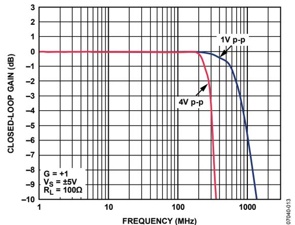
Figure 13. Large Signal Frequency Response vs. V<sub>OUT</sub> (LFCSP)
