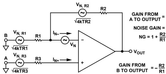
$$\blacklozenge \text{ RTI NOISE} = \sqrt{V_N^2 + 4kTR3 + 4kTR1 \left[ \frac{R2}{R1 + R2} \right]^2 + I_{N+}^2 R3^2 + I_{N-}^2 \left[ \frac{R1 \times R2}{R1 + R2} \right]^2 + 4kTR2 \left[ \frac{R1}{R1 + R2} \right]^2}$$
