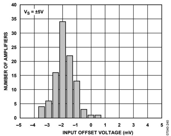
Figure 40. Input Offset Voltage Distribution,  $V_S = \pm 5 V$
