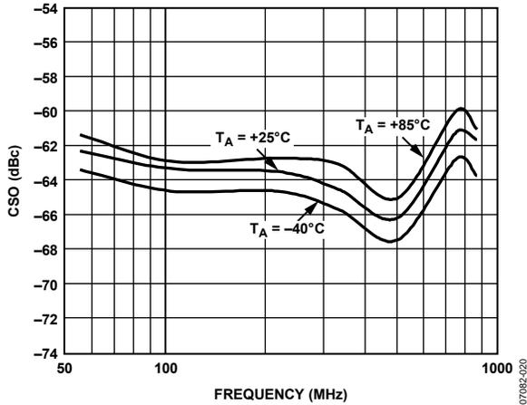
Figure 6. Composite Second Order (CSO) vs. Frequency
