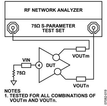
Figure 20. Test Circuit for Output-to-Output Isolation Measurements
