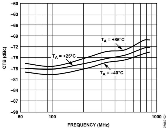
Figure 7. Composite Triple Beat (CTB) vs. Frequency
