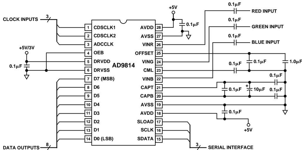
Figure 15. Recommended Circuit Configuration, 3-Channel CDS Mode
