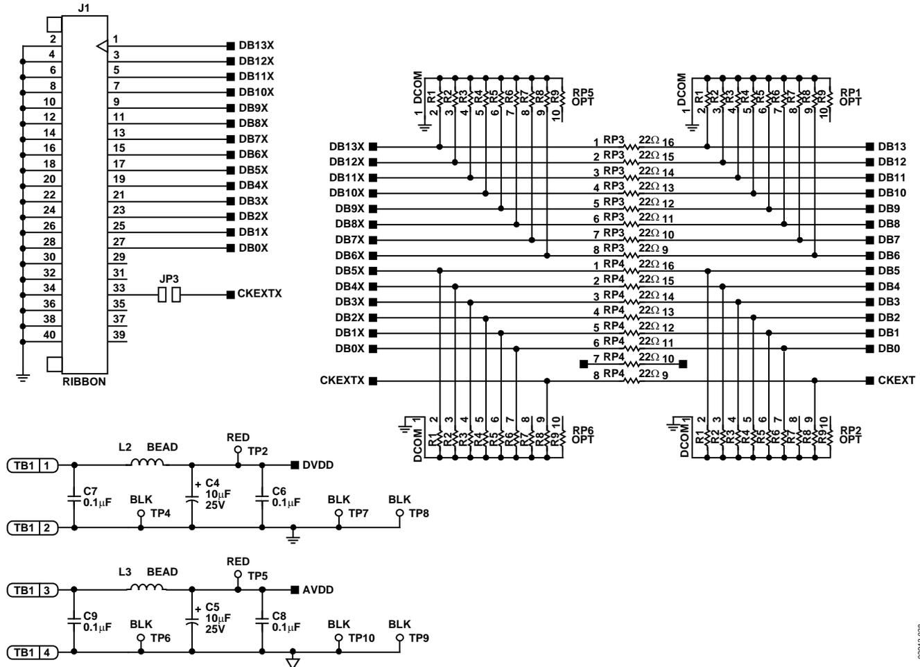
Figure 41. SOIC Evaluation Board—Power Supply and Digital Inputs
