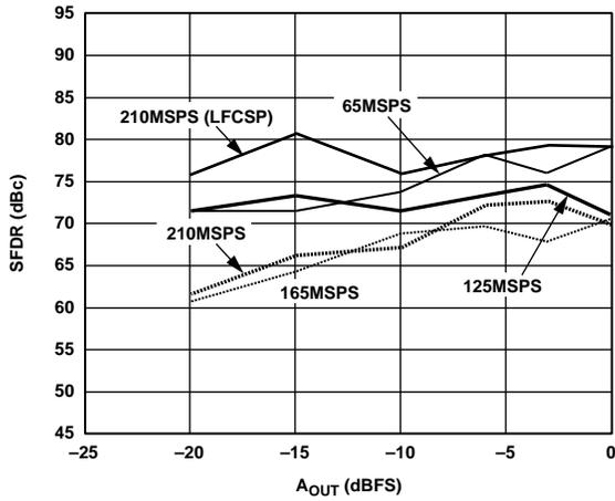
Figure 11. Single-Tone SFDR vs.  $A_{OUT}$  at  $f_{OUT} = f_{CLOCK}/11$
