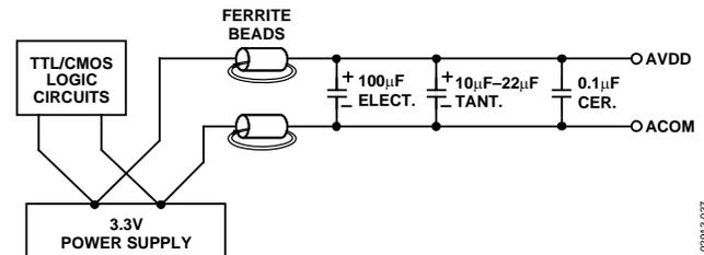
Figure 40. Differential LC Filter for Single 3.3 V Applications
