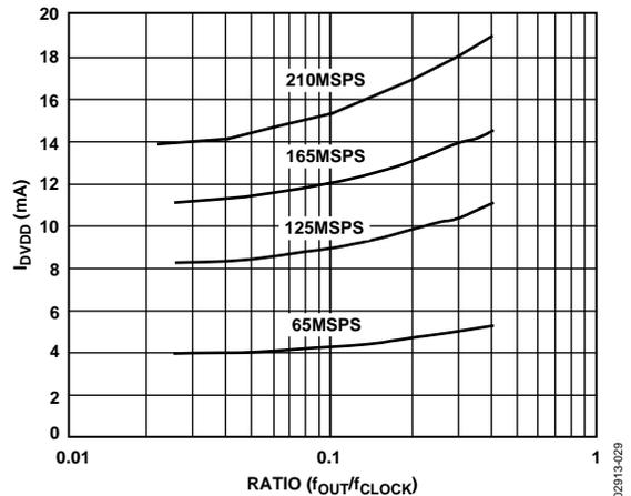
Figure 32.  $I_{DVDD}$  vs. Ratio at  $DVDD = 3.3\text{ V}$
