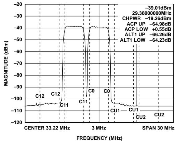
Figure 21. Two-Carrier UMTS Spectrum,  $f_{\text{CLOCK}} = 122.88 \text{ MSPS}$  (ACLR = 64 dB) LFCSP Package
