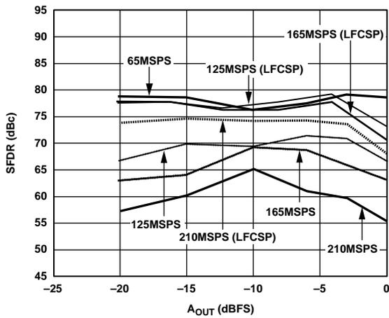
Figure 12. Single-Tone SFDR vs.  $A_{OUT}$  at  $f_{OUT} = f_{CLOCK}/5$
