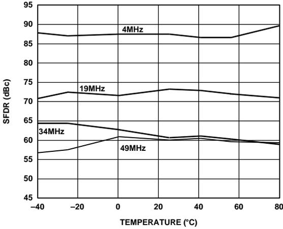
Figure 17. SFDR vs. Temperature at 165 MSPS, 0 dBFS
