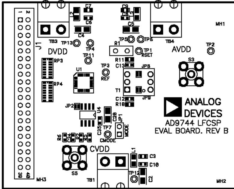
Figure 56. LFCSP Evaluation Board Layout Assembly—Primary Side
