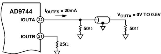
Figure 37. 0 V to 0.5 V Unbuffered Voltage Output
