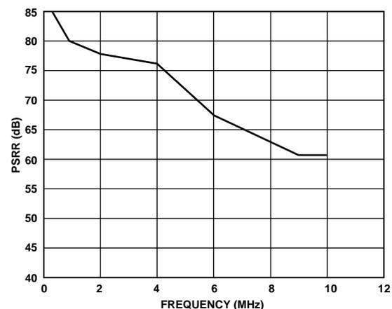
Figure 39. Power Supply Rejection Ratio (PSRR) vs. Frequency
