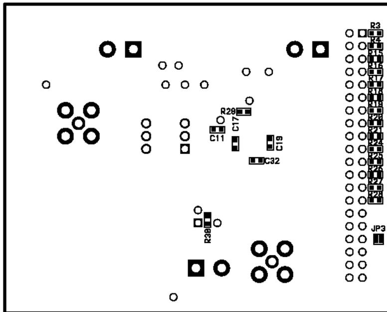
Figure 57. LFCSP Evaluation Board Layout Assembly—Secondary Side
