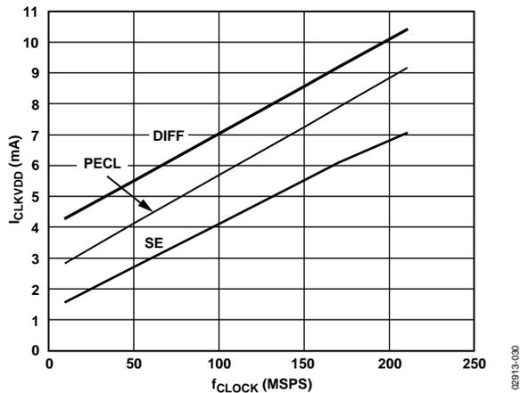
Figure 33.  $I_{CLKVDD}$  vs.  $f_{CLOCK}$  and Clock Mode
