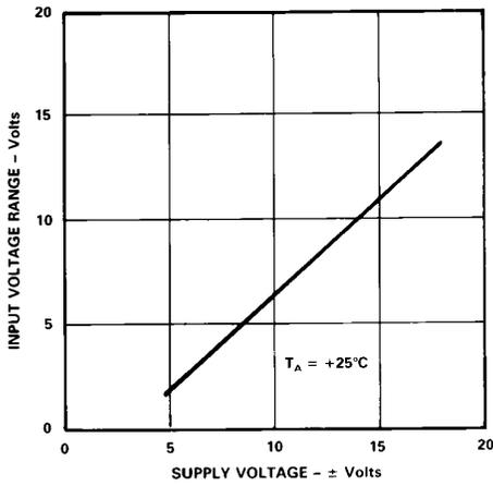
Figure 1. Input Voltage Range vs. Supply Voltage
