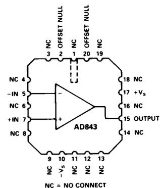
The AD843 is offered in either 8-pin plastic DIP or hermetic cerdip packages, in 16-pin SOIC, 20-Pin LCC, or in a 12-pin metal can. Chips are also available.
