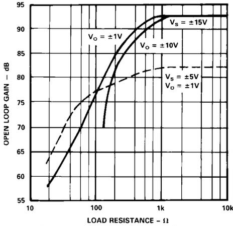
Figure 19. Open Loop Gain vs. Resistive Load
