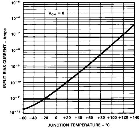
Figure 5. Input Bias Current vs. Junction Temperature
