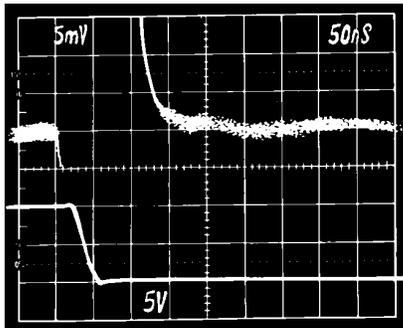
Figure 28. Settling Characteristics: +10 V to 0 V Step.
