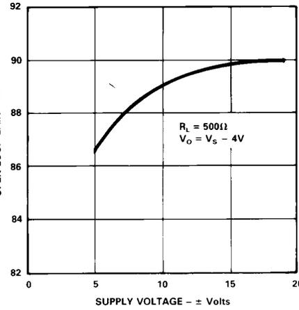
Figure 11. Open Loop Gain vs. Supply Voltage
