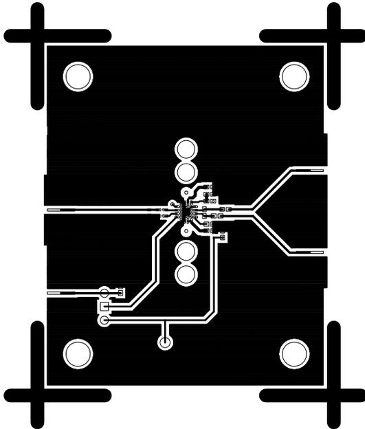
Figure 49. Component Side Layout
