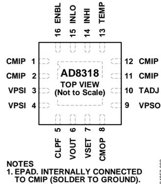
Figure 3. Pin Configuration
