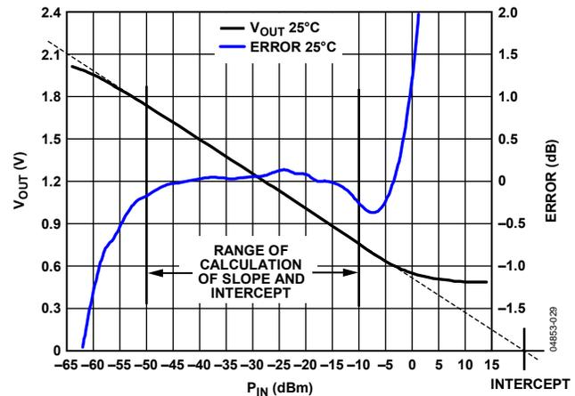
Figure 31. Typical Output Voltage vs. Input Signal
