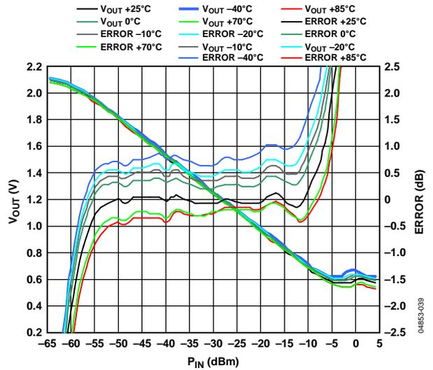
Figure 37. Typical Drift at 5.8 GHz for Various Temperatures
