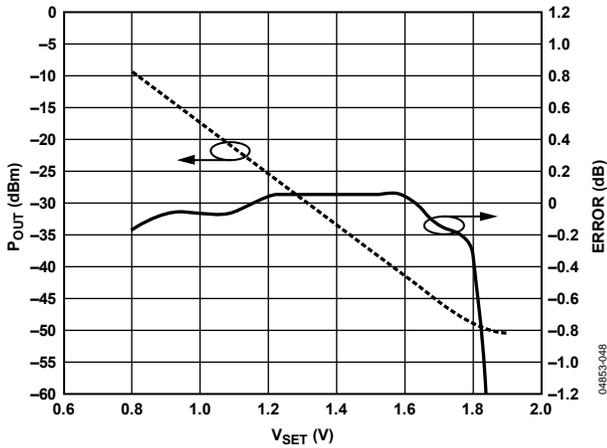
Figure 44. AD8367 Output Power vs. AD8318 Setpoint Voltage
