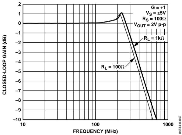
Figure 14. Large Signal Frequency Response for Various Loads
