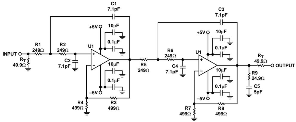
Figure 73. 4-Pole, 90 MHz, Sallen-Key Low-Pass Filter
