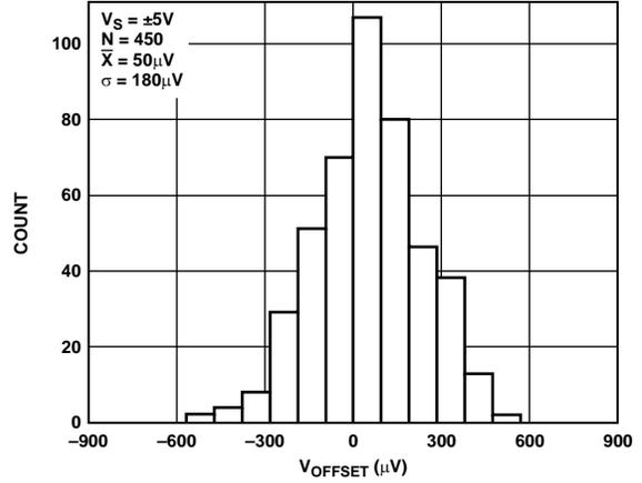
Figure 52.  $V_{OS}$  Distribution for  $V_S = \pm 5V$
