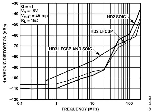
Figure 18. Harmonic Distortion vs. Frequency for Various Packages
