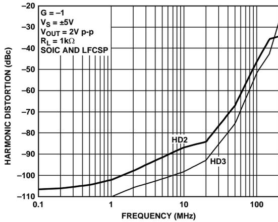
Figure 20. Harmonic Distortion vs. Frequency for Various Packages
