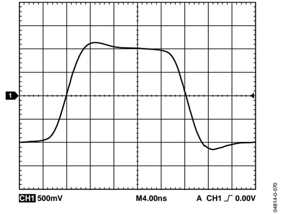
Figure 72. Large Signal Transient Response of 90 MHz LPF
