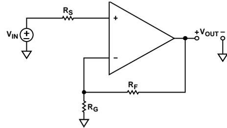
Figure 64. Noninverting Configuration
