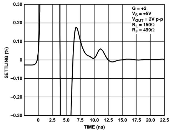
Figure 60. Short Term 0.1% Settling Time
