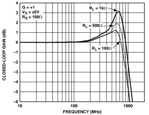
Figure 8. Small Signal Frequency Response for Various Loads
