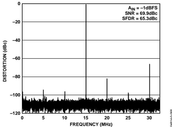
Figure 69. Single-Tone FFT,  $F_{IN} = 50$  MHz, Sample Rate = 65 MSPS
