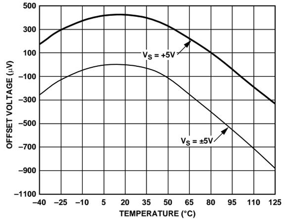
Figure 54. Offset Voltage vs. Temperature for Various Supplies
