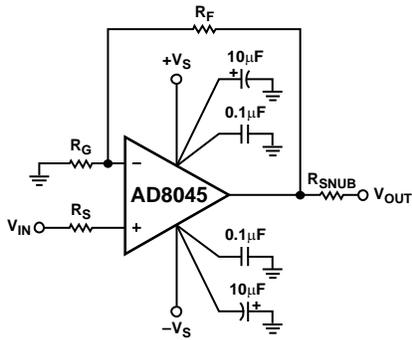
Figure 61. Noninverting Configuration
