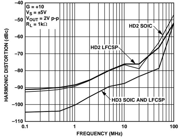
Figure 23. Harmonic Distortion vs. Frequency for Various Packages
