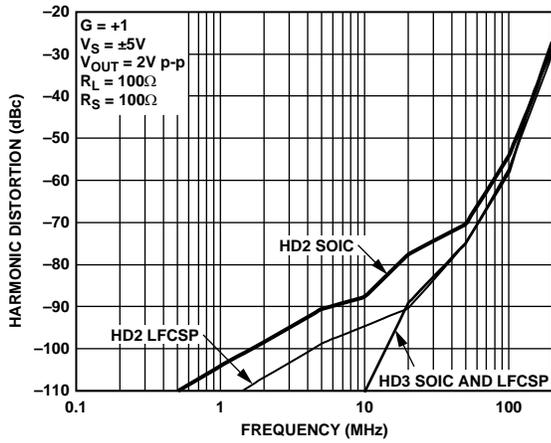
Figure 19. Harmonic Distortion vs. Frequency for Various Packages
