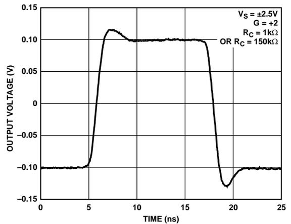
Figure 36. Small Signal Transient Response for Various Loads
