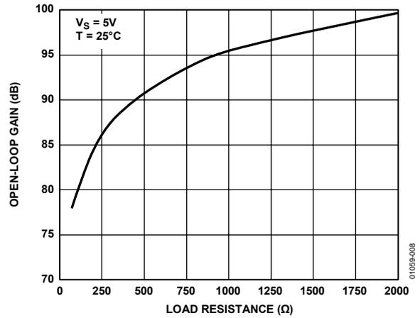
Figure 8. Open-Loop Gain vs.  $R_L$  to 2.5 V
