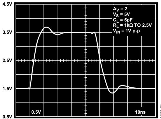
Figure 31. 1 V Pulse Response,  $V_S = 5V$
