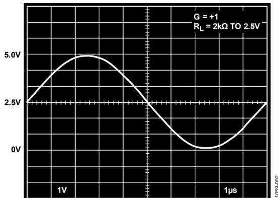
Figure 1. Output Swing: Gain = +1,  $V_S = +5$  V
