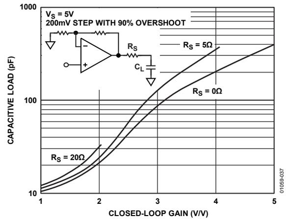
Figure 36. Capacitive Load Drive vs. Closed-Loop Gain
