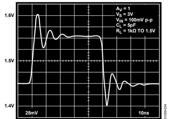
Figure 34. 100 mV Pulse Response,  $V_S = 3V$
