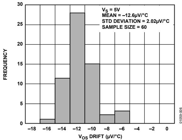
Figure 6.  $V_{OS}$  Drift Over  $-40^{\circ}\text{C}$  to  $+85^{\circ}\text{C}$
