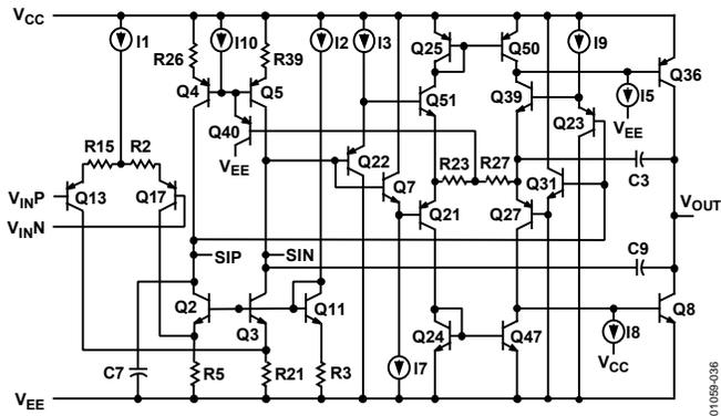
Figure 35. Simplified Schematic
