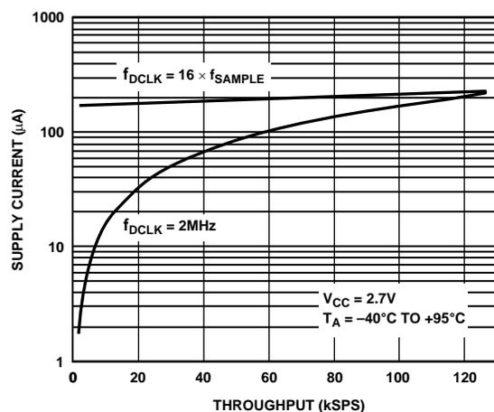
Figure 23. Supply Current vs. Throughput ( $\mu\text{A}$ )
