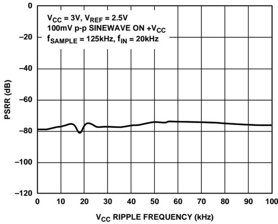
Figure 16. AC PSRR vs. Supply Ripple Frequency
