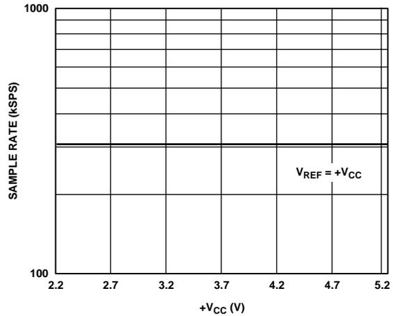
Figure 8. Maximum Sample Rate vs. +V<sub>CC</sub>
