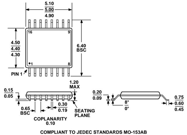
Figure 31. 16-Lead Thin Shrink Small Outline Package [TSSOP]
