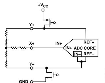
Figure 22. Differential Reference Mode ( $\overline{\text{SER/DFR}} = 0$ )
