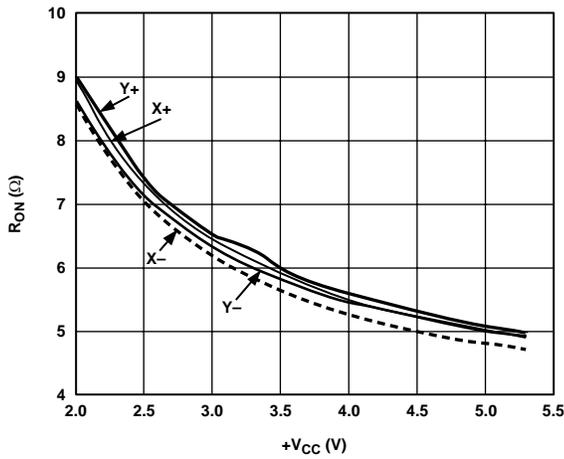
Figure 11. Switch-On Resistance vs. +Vcc
