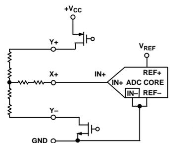
Figure 21. Single-Ended Reference Mode ( $\overline{\text{SER/DFR}} = 1$ )
