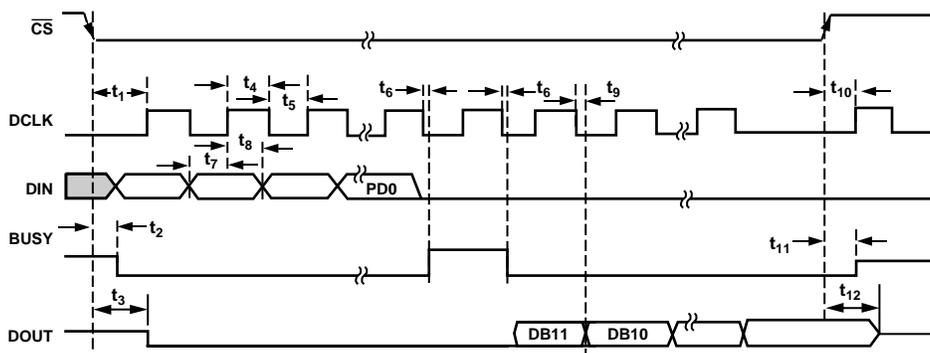
Figure 25. Detailed Timing Diagram
