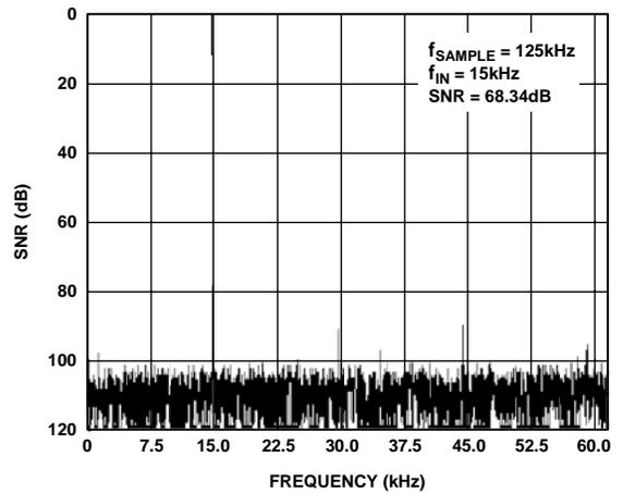
Figure 15. Auxiliary Channel Dynamic Performance
