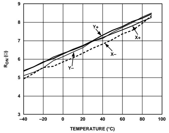
Figure 14. Switch-On Resistance vs. Temperature
