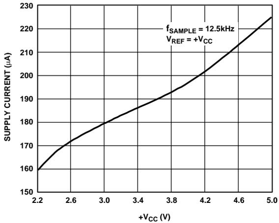
Figure 5. Supply Current vs. +V<sub>CC</sub>
