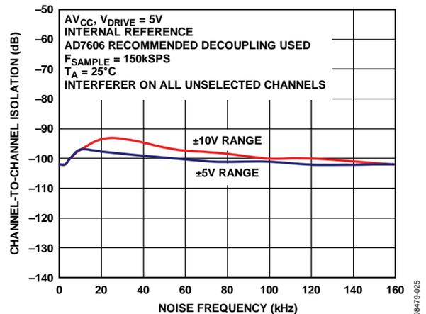
Figure 28. Channel-to-Channel Isolation
