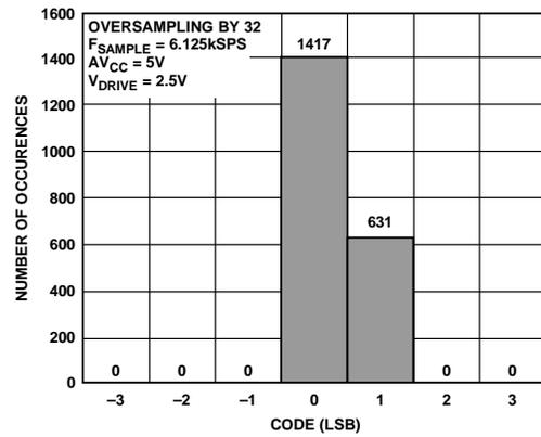
Figure 54. Histogram of Codes—OS x 32 (Two Codes)
