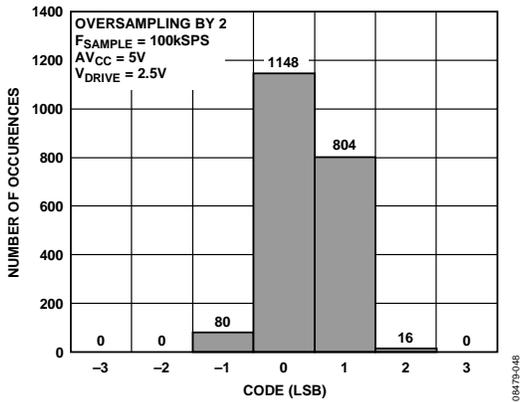
Figure 50. Histogram of Codes—OS x 2 (Four Codes)
