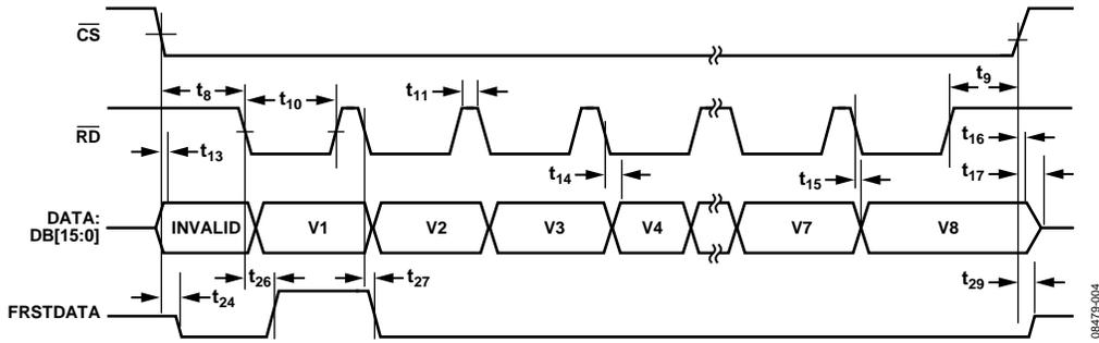
Figure 4. Parallel Mode, Separate  $\overline{CS}$  and  $\overline{RD}$  Pulses
