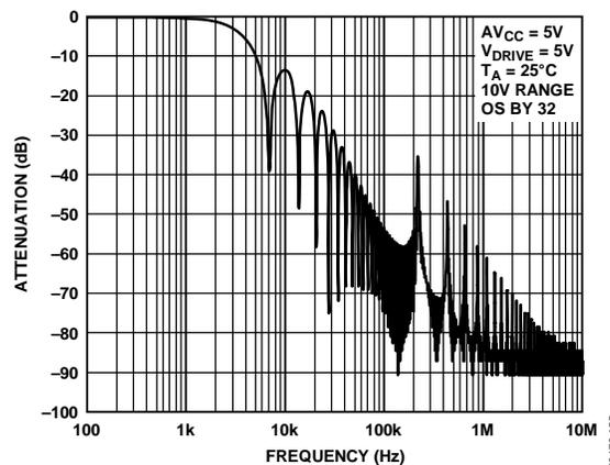
Figure 60. Digital Filter Response for OS 32
