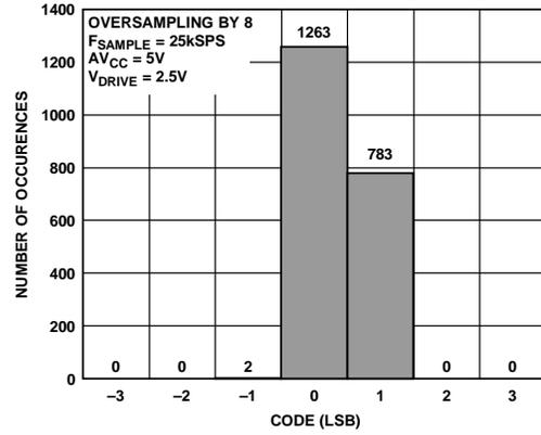
Figure 52. Histogram of Codes—OS x 8 (Three Codes)
