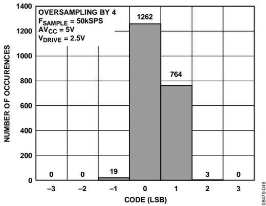
Figure 51. Histogram of Codes—OS x 4 (Four Codes)
