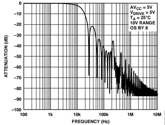
Figure 58. Digital Filter Response for OS 8
