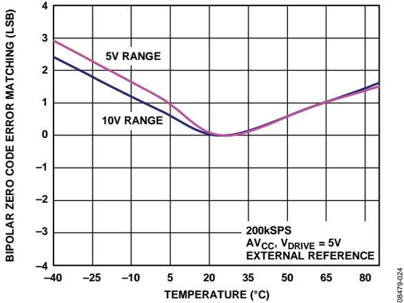
Figure 23. Bipolar Zero Code Error Matching Between Channels
