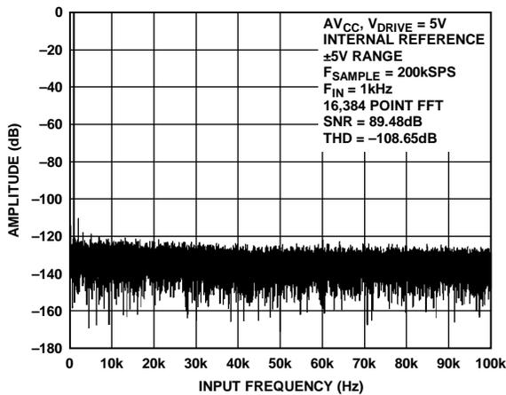
Figure 12. AD7606 FFT Plot,  $\pm 5$  V Range
