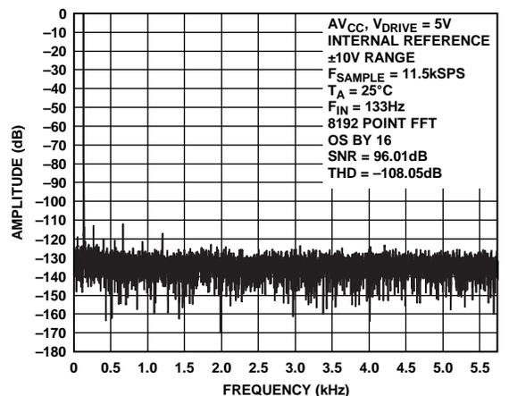
Figure 13. FFT Plot Oversampling By 16,  $\pm 10$  V Range
