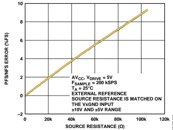
Figure 21. PFS and NFS Error vs. Source Resistance
