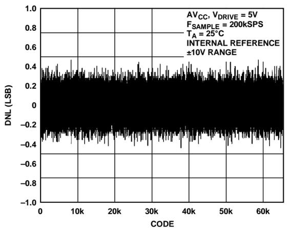
Figure 15. AD7606 Typical DNL,  $\pm 10$  V Range
