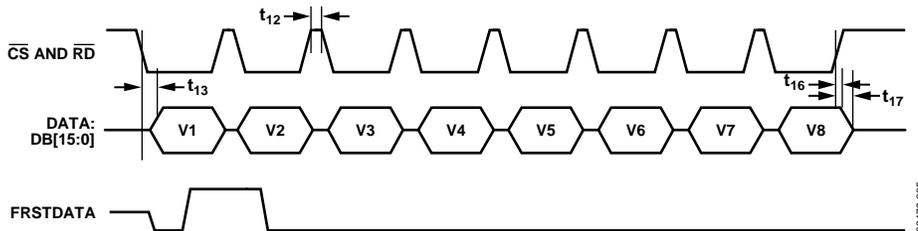
Figure 5.  $\overline{CS}$  and  $\overline{RD}$ , Linked Parallel Mode
