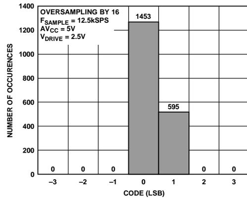
Figure 53. Histogram of Codes—OS x 16 (Two Codes)
