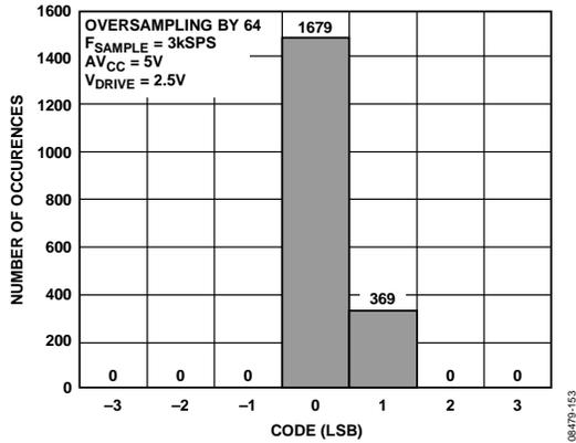
Figure 55. Histogram of Codes—OS x 64 (Two Codes)
