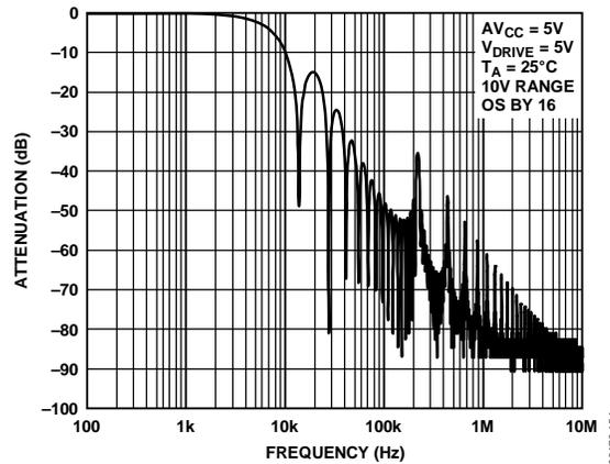
Figure 59. Digital Filter Response for OS 16
