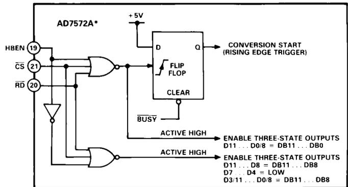
\*NOTE: D11...D0/8 ARE THE ADC DATA OUTPUT PINS.
