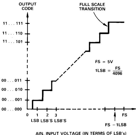
Figure 8. AD7572A Ideal Input/Output Transfer Characteristic
