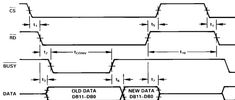
Figure 17. Slow Memory Mode, Parallel Read Timing Diagram
