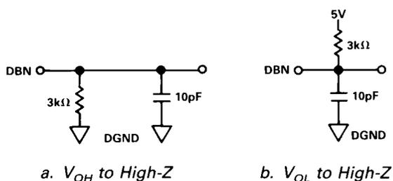
Figure 2. Load Circuits for Output Float Delay
