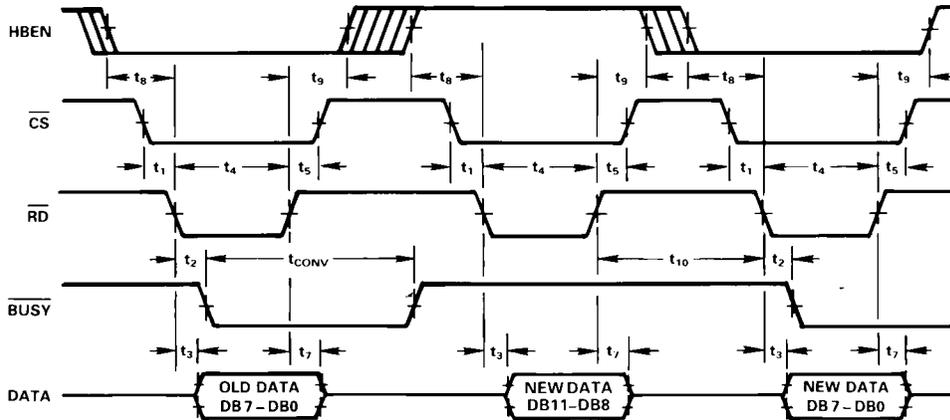
Figure 20. ROM Mode, Two Byte Read Timing Diagram
