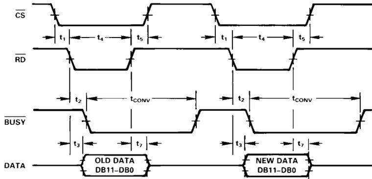
Figure 19. ROM Mode, Parallel Read Timing Diagram
