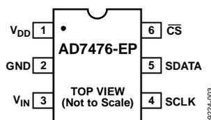
Figure 3. Pin Configuration
