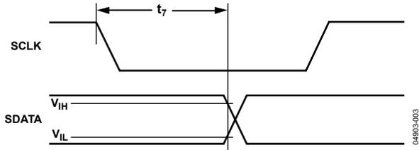
Figure 3. Hold Time After SCLK Falling Edge
