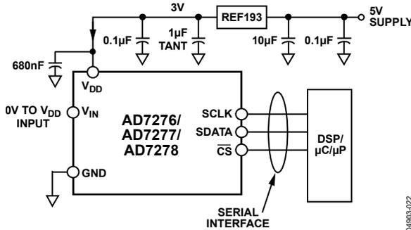
Figure 22. REF193 as Power Supply to the AD7276/AD7277/AD7278
