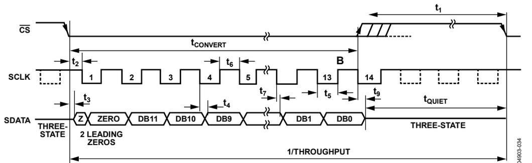
Figure 6. AD7276 Serial Interface Timing 14 SCLK Cycle
