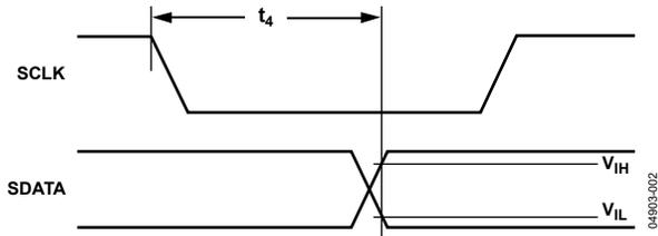
Figure 2. Access Time After SCLK Falling Edge
