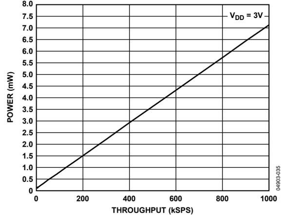
Figure 30. Power vs. Throughput Partial Power-Down Mode
