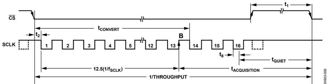
Figure 7. AD7276 Serial Interface Timing 16 SCLK Cycle
