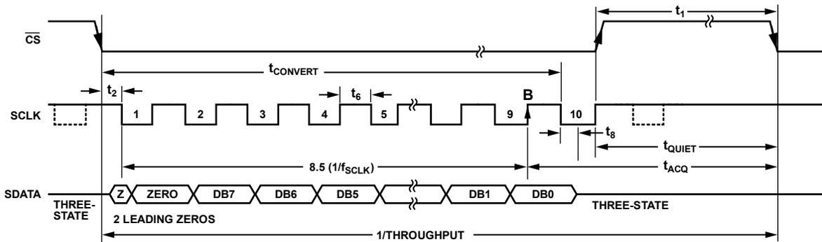
Figure 35. AD7278 in a 10 SCLK Cycle Serial Interface
