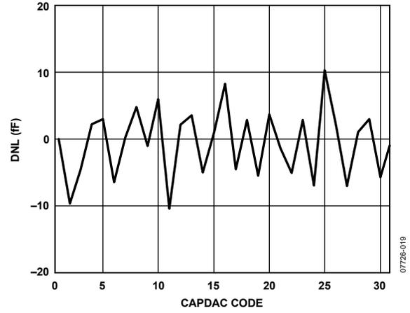
Figure 19. CAPDAC Differential Nonlinearity (DNL),  $V_{DD} = 1.8\text{ V}$
