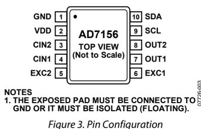
Figure 3. Pin Configuration
