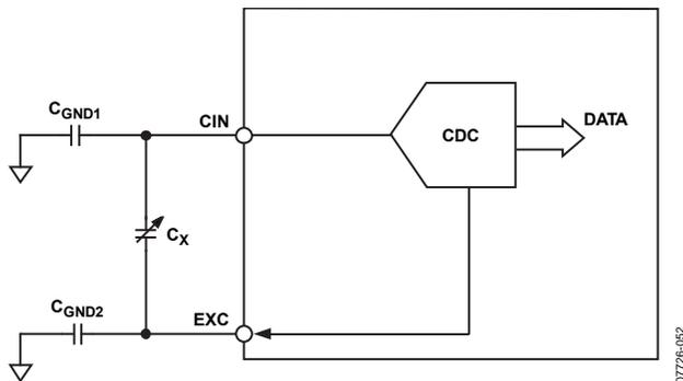
Figure 42. Parasitic Capacitance to Ground
