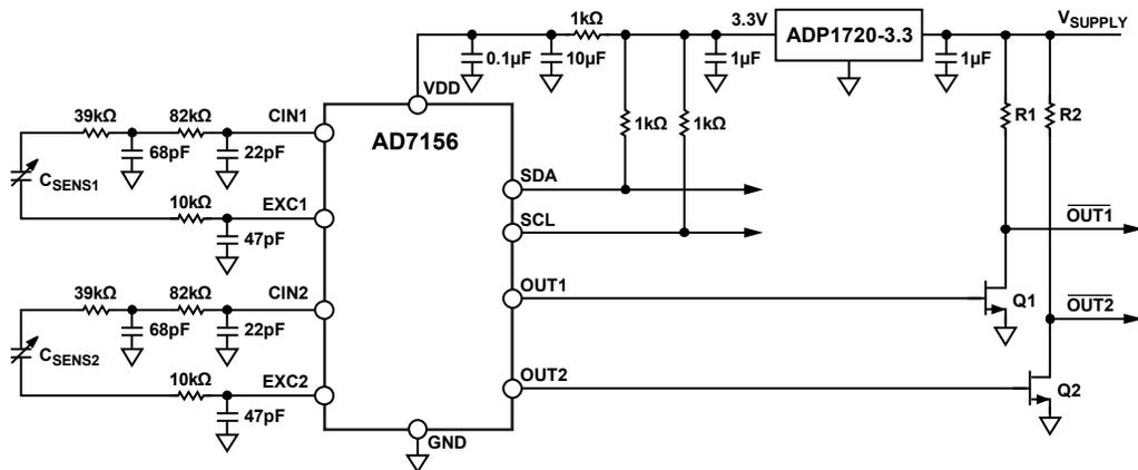
Figure 51. AD7156 Standalone Operation with EMC Protection
