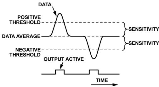
Figure 37. Threshold Sensitivity
