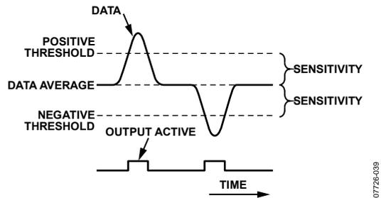
Figure 30. Threshold Sensitivity
