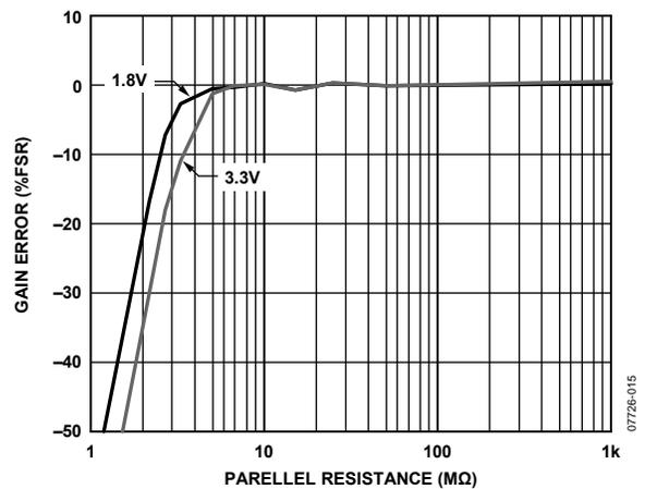
Figure 15. Capacitance Input Gain Error vs. Parallel Resistance,  $V_{DD} = 1.8\text{ V}$  and  $3.3\text{ V}$ ,  $C_{IN}$  to  $C_{EXC} = 3\text{ pF}$
