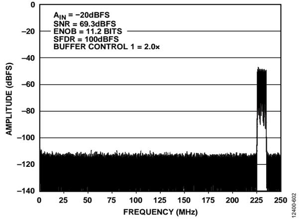
Figure 53. LTE-TDD 10 MHz Channel FFT with  $f_{IN} = 230$  MHz
