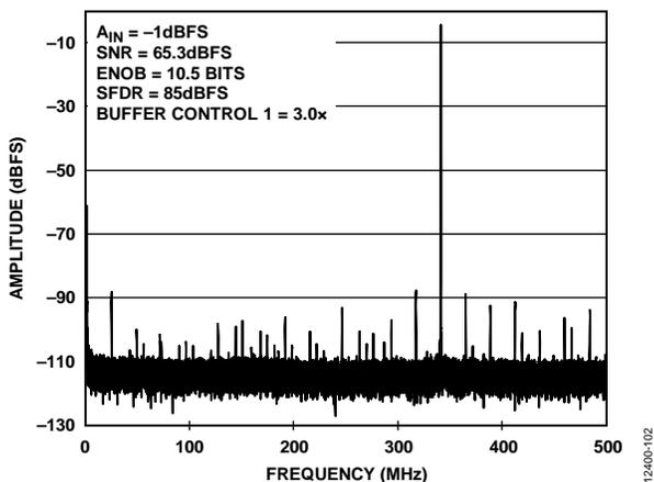
Figure 8. Single Tone FFT with  $f_{IN} = 340.3$  MHz
