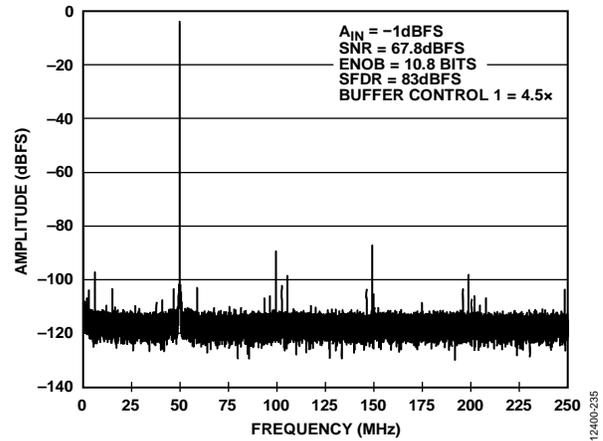
Figure 47. Single Tone FFT with  $f_{IN} = 450.3$  MHz
