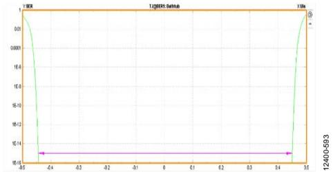
Figure 134. Bathtub, External 100Ω Terminations at 7.37 Gbps
