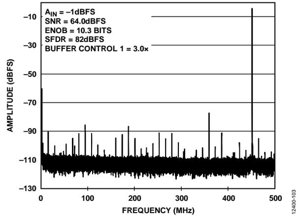
Figure 9. Single Tone FFT with  $f_{IN} = 450.3$  MHz
