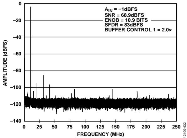
Figure 44. Single Tone FFT with  $f_{IN} = 10.3$  MHz
