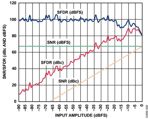
Figure 41. SNR/SFDR vs. Input Amplitude ( $A_{IN}$ ),  $f_{IN} = 170.3$  MHz
