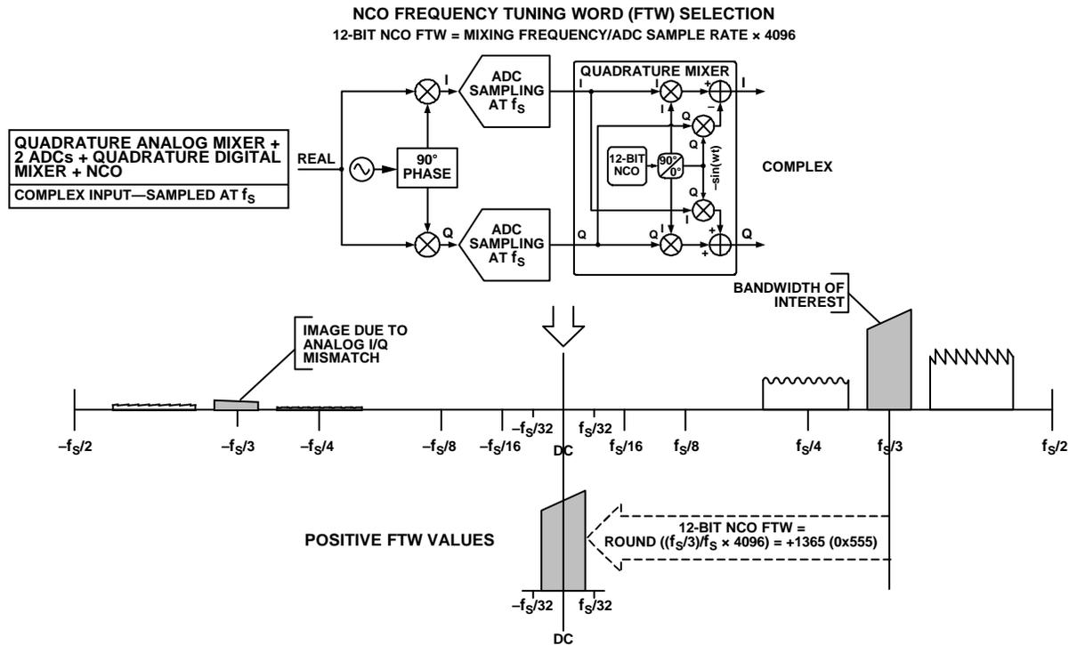
Figure 105. DDC NCO Frequency Tuning Word Selection—Complex Inputs
