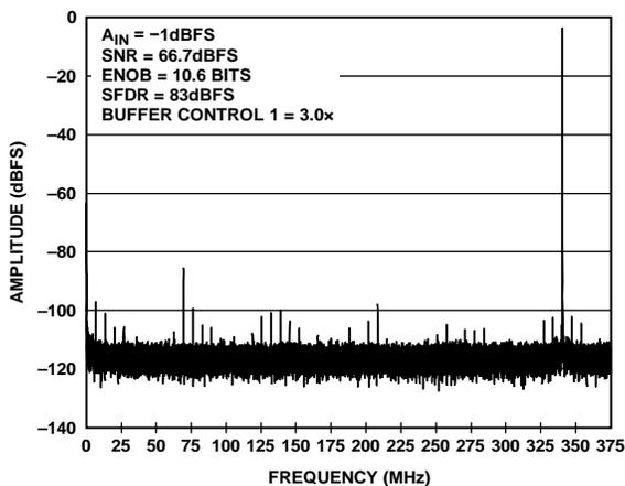
Figure 27. Single Tone FFT with  $f_{IN} = 340.3$  MHz
