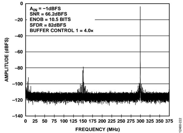
Figure 28. Single Tone FFT with  $f_{IN} = 450.3$  MHz
