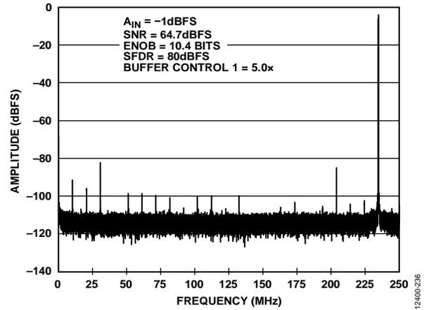
Figure 48. Single Tone FFT with  $f_{IN} = 765.3$  MHz
