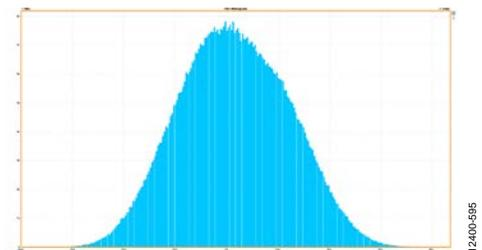
Figure 136. Histogram, External 100Ω Terminations at 6 Gbps
