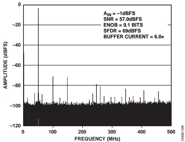
Figure 14. Single Tone FFT with  $f_{IN} = 1950.3$  MHz
