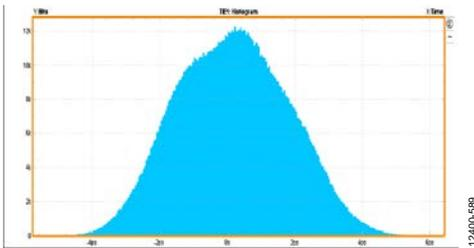
Figure 130. Histogram, External 100Ω Terminations at 10 Gbps
