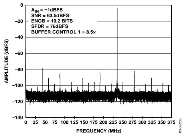
Figure 30. Single Tone FFT with  $f_{IN} = 985.3$  MHz
