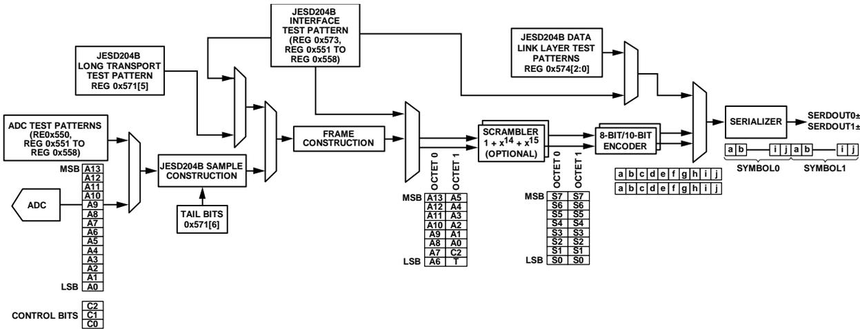
Figure 124. ADC Output Datapath Showing Data Framing
