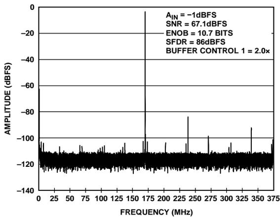
Figure 26. Single Tone FFT with  $f_{IN} = 170.3$  MHz
