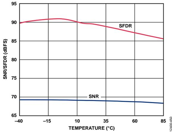
Figure 61. SNR/SFDR vs. Temperature,  $f_{IN} = 170.3$  MHz
