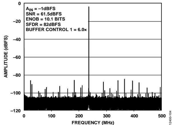
Figure 10. Single Tone FFT with  $f_{IN} = 765.3$  MHz
