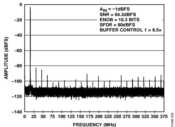
Figure 29. Single Tone FFT with  $f_{IN} = 765.3$  MHz
