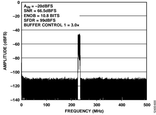
Figure 15. LTE-FDD 10 MHz Channel FFT with  $f_{IN} = 230$  MHz
