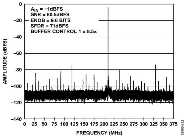
Figure 32. Single Tone FFT with  $f_{IN} = 1710.3$  MHz
