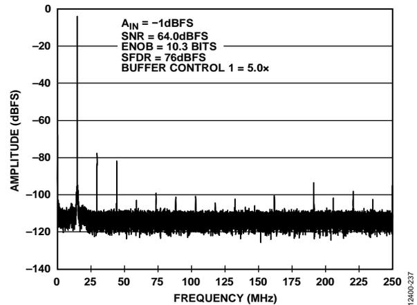
Figure 49. Single Tone FFT with  $f_{IN} = 985.3$  MHz
