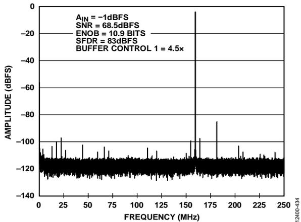
Figure 46. Single Tone FFT with  $f_{IN} = 340.3$  MHz
