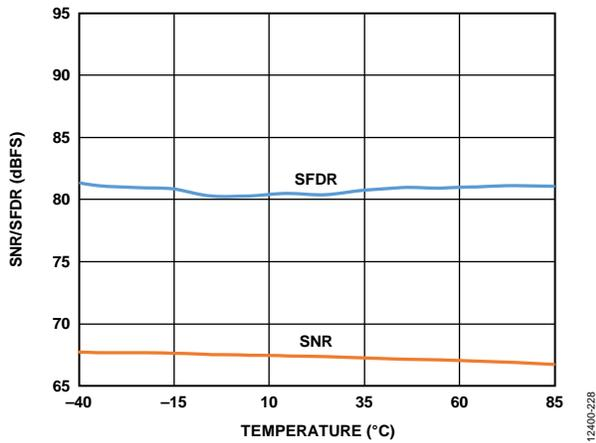
Figure 42. SNR/SFDR vs. Temperature,  $f_{IN} = 170.3$  MHz
