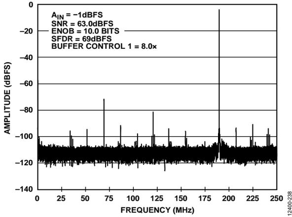
Figure 50. Single Tone FFT with  $f_{IN} = 1310.3$  MHz
