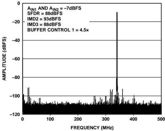
Figure 19. Two-Tone FFT;  $f_{IN1} = 338$  MHz,  $f_{IN2} = 341$  MHz
