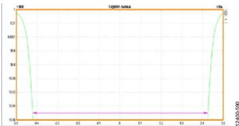
Figure 131. Bathtub, External 100Ω Terminations at 10 Gbps
