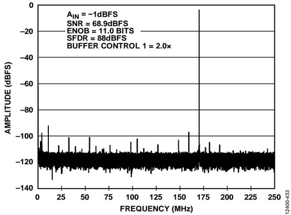
Figure 45. Single Tone FFT with  $f_{IN} = 170.3$  MHz
