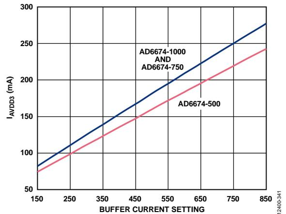
Figure 76. I<sub>AVDD3</sub> vs. Buffer Current Setting in Register 0x018
