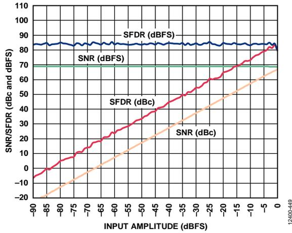
Figure 60. SNR/SFDR vs. Input Amplitude ( $A_{IN}$ ),  $f_{IN} = 170.3$  MHz
