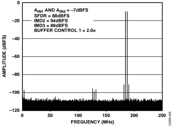
Figure 56. Two-Tone FFT;  $f_{IN1} = 184$  MHz,  $f_{IN2} = 187$  MHz
