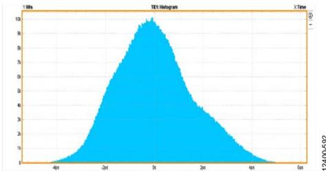
Figure 133. Histogram, External 100Ω Terminations at 7.37 Gbps
