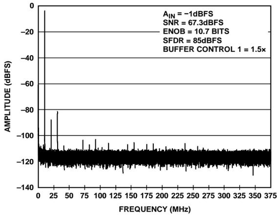
Figure 25. Single Tone FFT with  $f_{IN} = 10.3$  MHz
