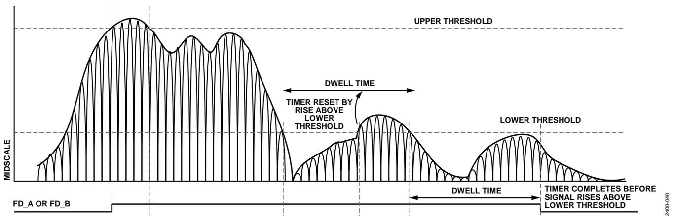
Figure 97. Threshold Settings for FD\_A and FD\_B Signals
