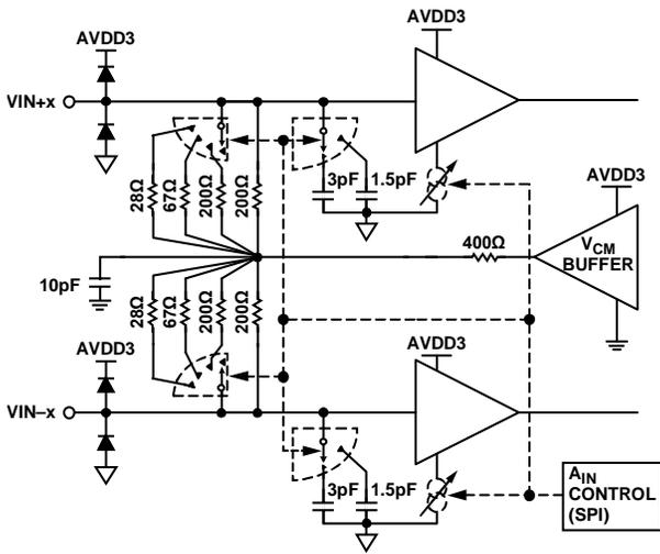
Figure 63. Analog Inputs
