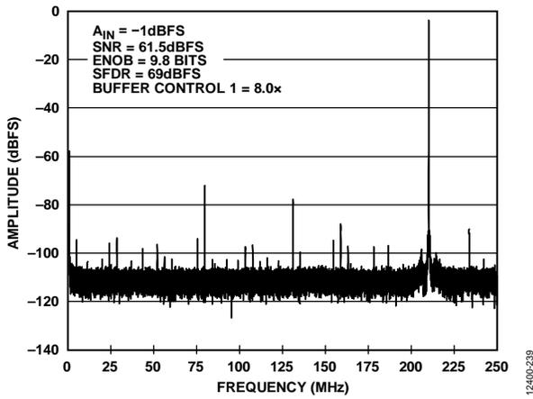
Figure 51. Single Tone FFT with  $f_{IN} = 1710.3$  MHz
