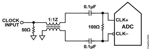
Figure 90. Transformer Coupled Differential Clock
