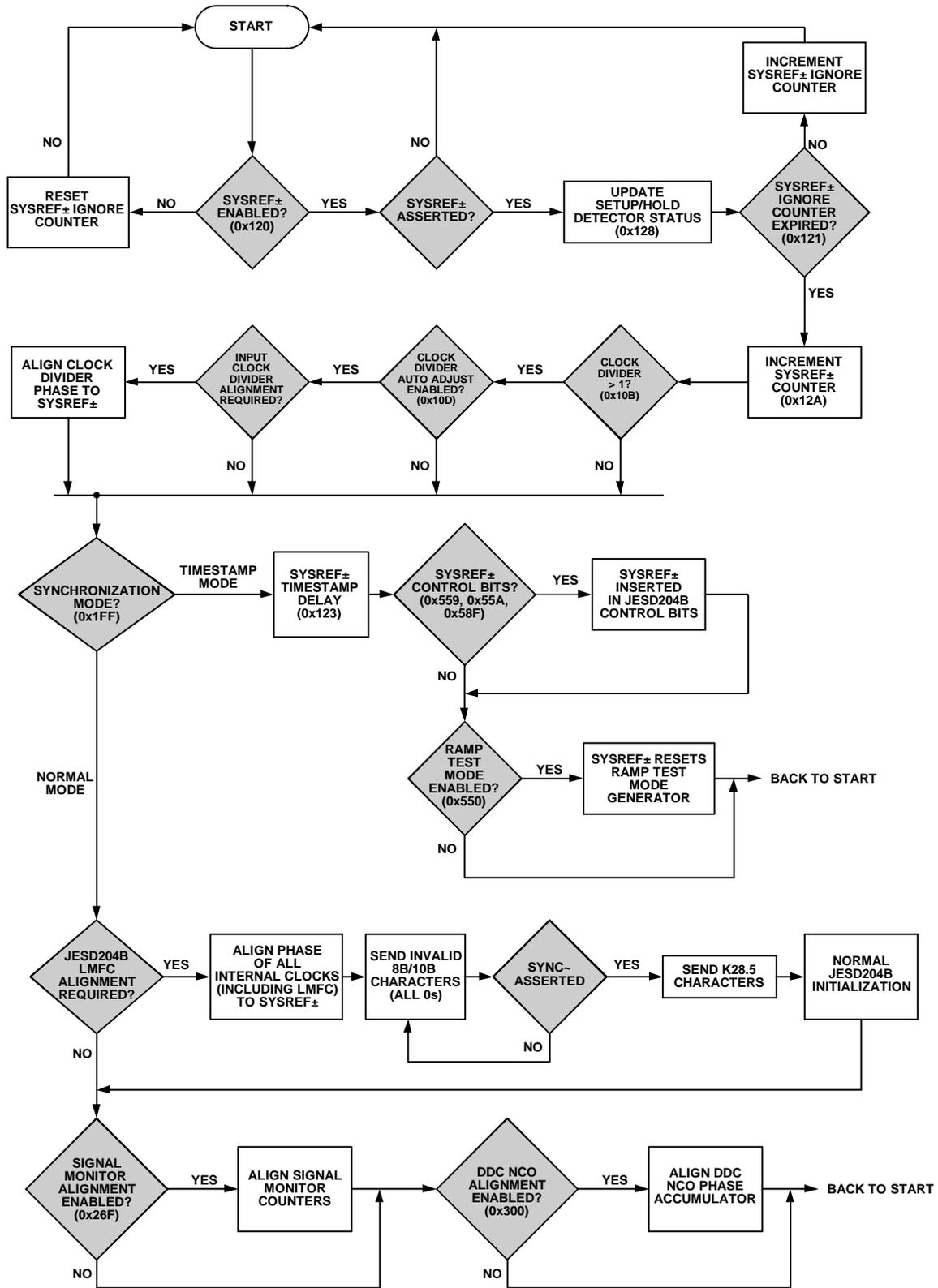
Figure 142. Multichip Synchronization
