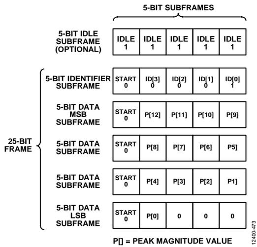
Figure 100. SPORT over JESD204B Signal Monitor Frame Data
