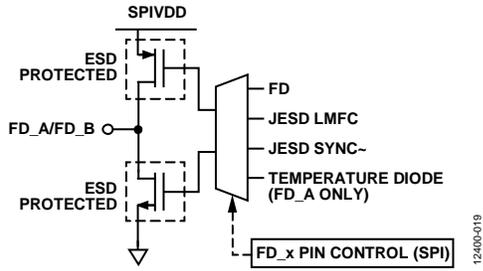
Figure 71. FD\_A/FD\_B Outputs
