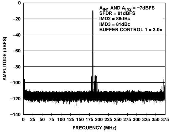
Figure 37. Two-Tone FFT;  $f_{IN1} = 184$  MHz,  $f_{IN2} = 187$  MHz
