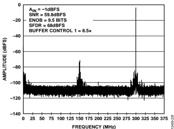
Figure 33. Single Tone FFT with  $f_{IN} = 1950.3$  MHz
