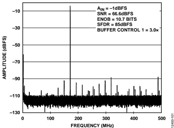
Figure 7. Single Tone FFT with  $f_{IN} = 170.3$  MHz
