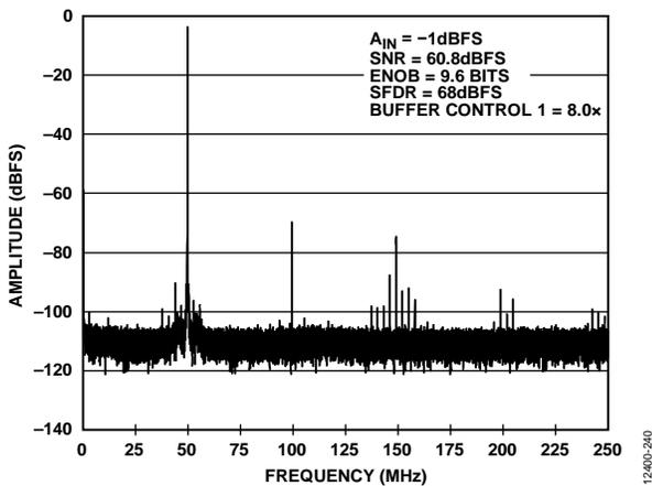
Figure 52. Single Tone FFT with  $f_{IN} = 1950.3$  MHz
