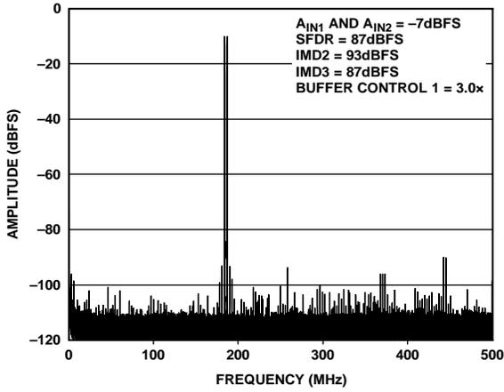
Figure 18. Two-Tone FFT;  $f_{IN1} = 184$  MHz,  $f_{IN2} = 187$  MHz
