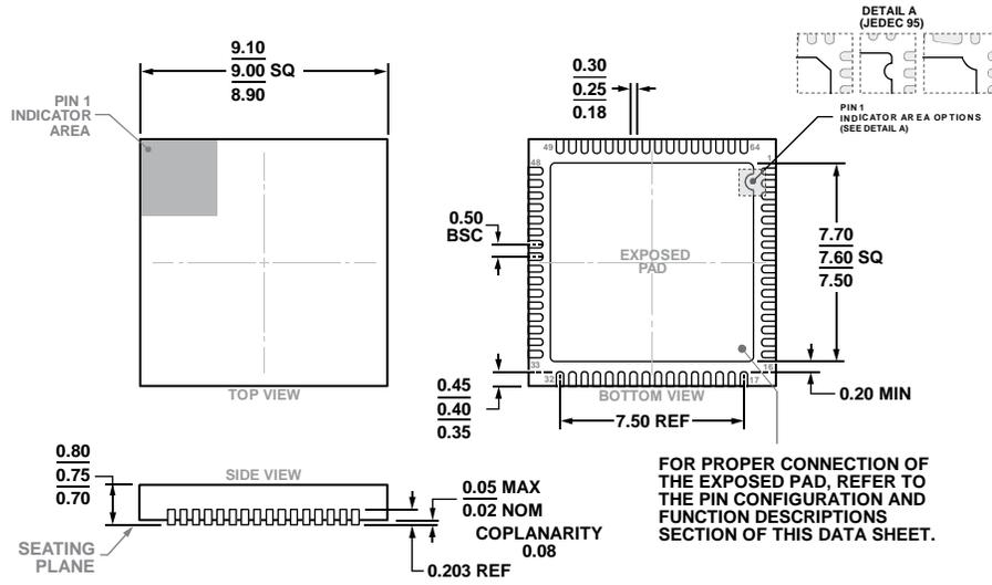
Figure 147. 64-Lead Lead Frame Chip Scale Package [LFCSP]
