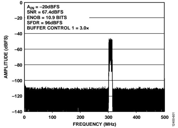
Figure 34. LTE-FDD 10 MHz Channel FFT with  $f_{IN} = 230$  MHz
