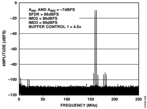
Figure 57. Two-Tone FFT;  $f_{IN1} = 338$  MHz,  $f_{IN2} = 341$  MHz
