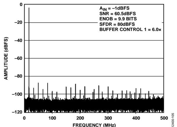
Figure 11. Single Tone FFT with  $f_{IN} = 985.3$  MHz
