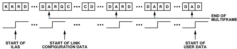
Figure 126. Initial Lane Alignment Sequence
