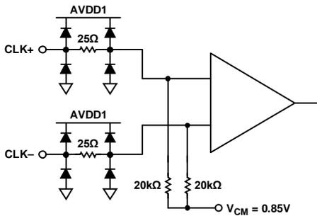
Figure 64. Clock Inputs
