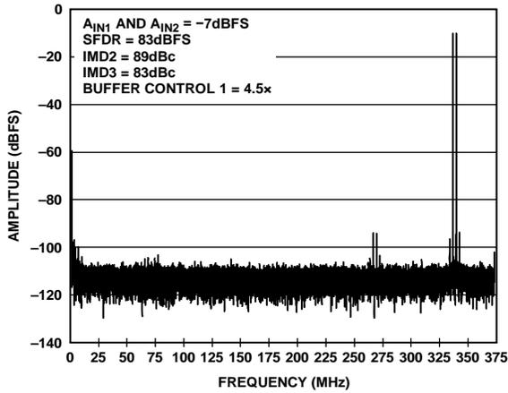
Figure 38. Two-Tone FFT;  $f_{IN1} = 338$  MHz,  $f_{IN2} = 341$  MHz
