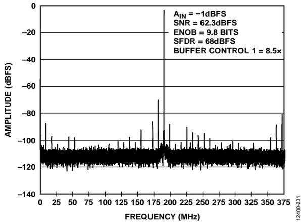
Figure 31. Single Tone FFT with  $f_{IN} = 1310.3$  MHz
