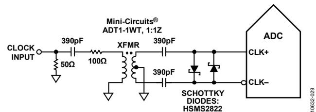
Figure 33. Transformer-Coupled Differential Clock (Up to 200 MHz)
