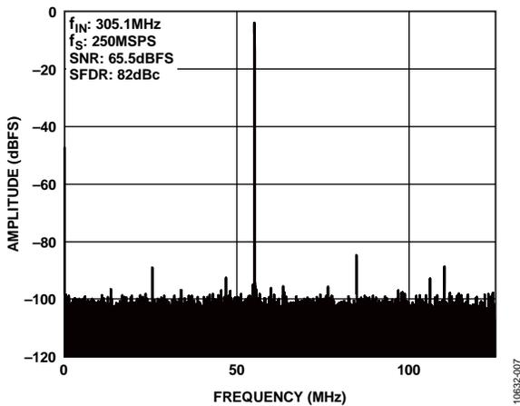
Figure 7. AD6673-250 Single-Tone FFT with  $f_{IN} = 305.1$  MHz
