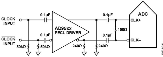
Figure 35. Differential PECL Sample Clock (Up to 625 MHz)
