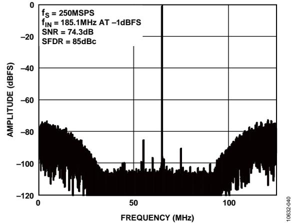
Figure 44. 22% Bandwidth Mode, Tuning Word = 28 ( $f_c/4$  Tuning)
