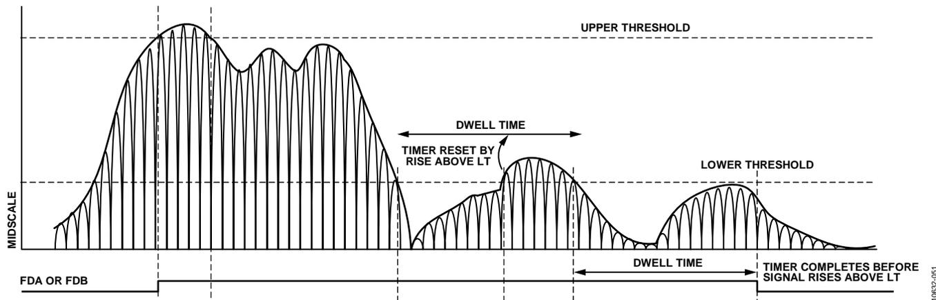
Figure 55. Threshold Settings for FDA and FDB Signals
