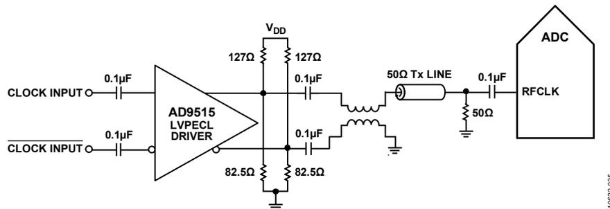
Figure 39. Differential PECL RF Clock Input Circuit
