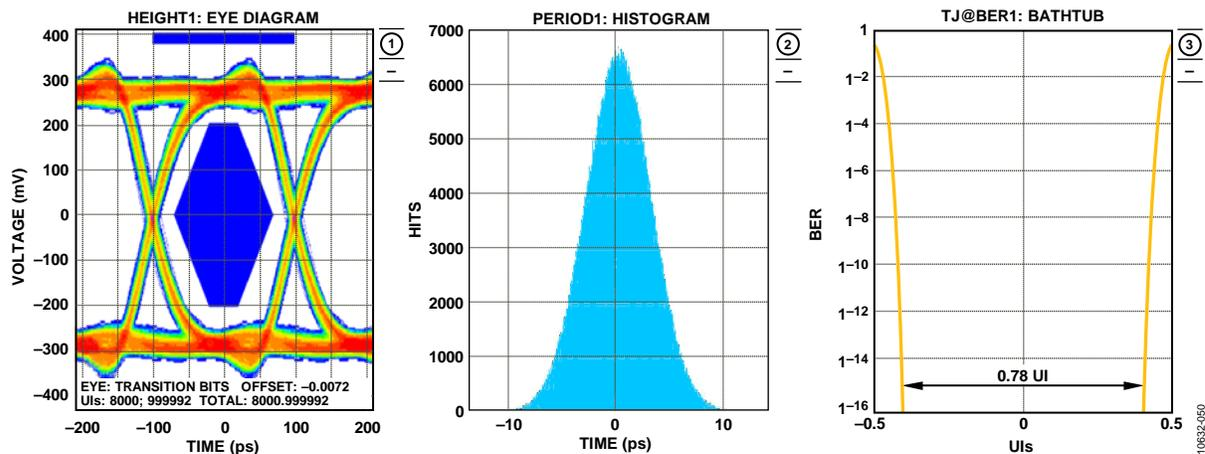
Figure 54. AD6673 Digital Outputs Data Eye, Histogram, and Bathtub, External 100  $\Omega$  Terminations at 5 Gbps
