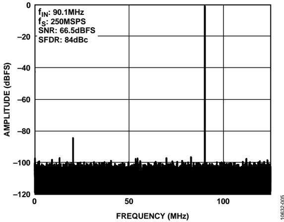
Figure 5. AD6673-250 Single-Tone FFT with  $f_{IN} = 90.1$  MHz
