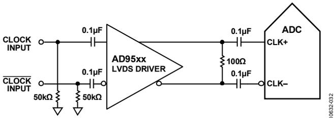
Figure 36. Differential LVDS Sample Clock (Up to 625 MHz)
