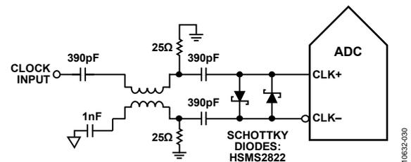
Figure 34. Balun-Coupled Differential Clock (Up to 625 MHz)
