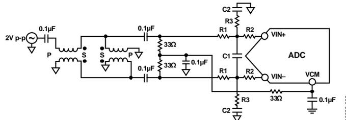
Figure 30. Differential Double Balun Input Configuration
