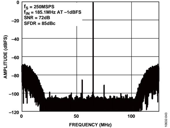
Figure 47. 33% Bandwidth Mode, Tuning Word = 17 ( $f_s/4$  Tuning)
