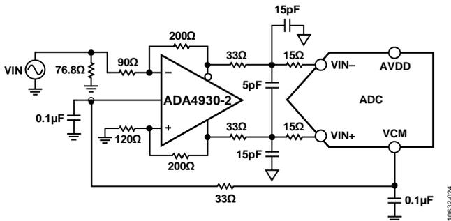
Figure 28. Differential Input Configuration Using the ADA4930-2
