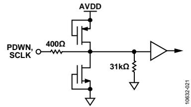
Figure 21. Equivalent SCLK or PDWN Input Circuit
