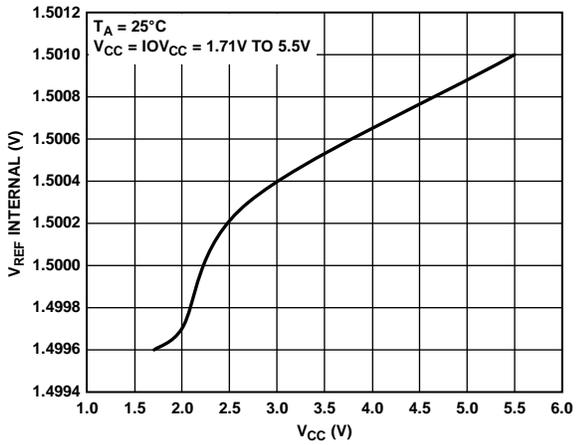
Figure 15. Reference Voltage vs.  $V_{CC}$
