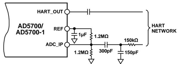
Figure 23. AD5700/AD5700-1 with External Filter on ADC\_IP
