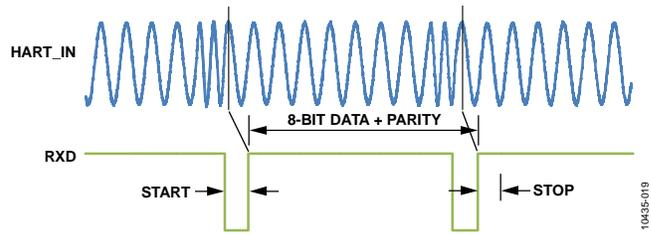
Figure 22. AD5700/AD5700-1 Demodulator Waveform (Preamble Message 0xFF)
