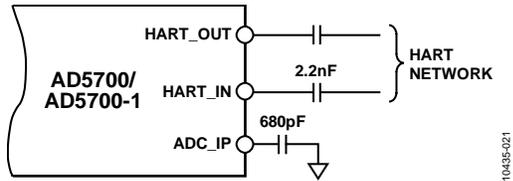
Figure 24. AD5700/AD5700-1 Using Internal Filter on HART\_IN
