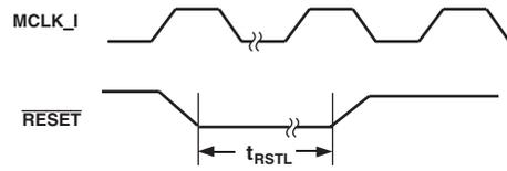
Figure 2. RESET Timing
