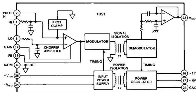
the front end and a two-pole active filter at the output. Overall NMR is 60dB and CMR is 160dB min @ 60Hz,  $G=1000$ .
