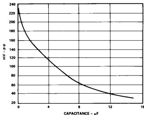
+V<sub>ISO</sub> Ripple vs. Capacitance
