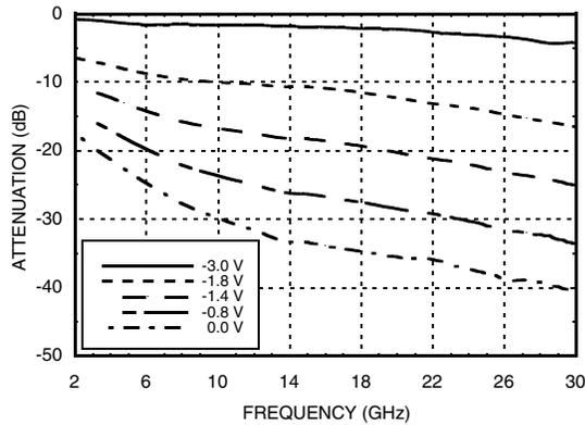
**Attenuation vs. Vctrl over Temperature
