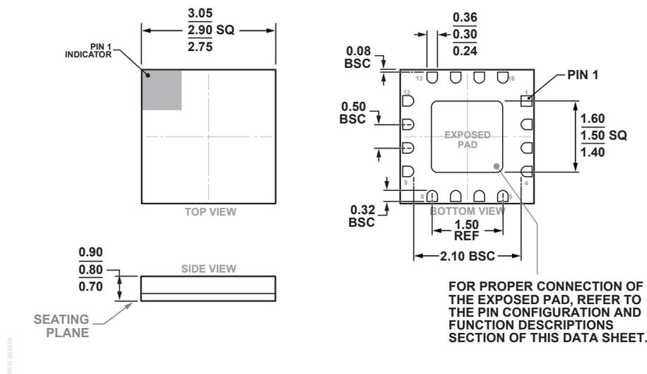
16-Terminal Ceramic Leadless Chip Carrier [LCC]
