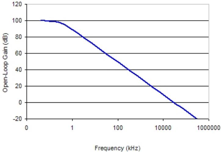
The idealized open loop gain plot is provided for information only. This information is associated with the dpASP in full power mode of operation. The dpASP operational amplifier open loop gain cannot be observed nor used when associated with external connections to the device. Internal reprogrammable routing impedances and switched capacitor circuit architectures using this operational amplifier limit the effective usable bandwidth.
