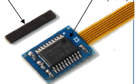
**TRK-1T02-E Evaluation Pack** includes an NSE5310 in a TSSOP 20 package on a board for ease of handling, along with a matching linear magnetic strip. See page 2 for details.
