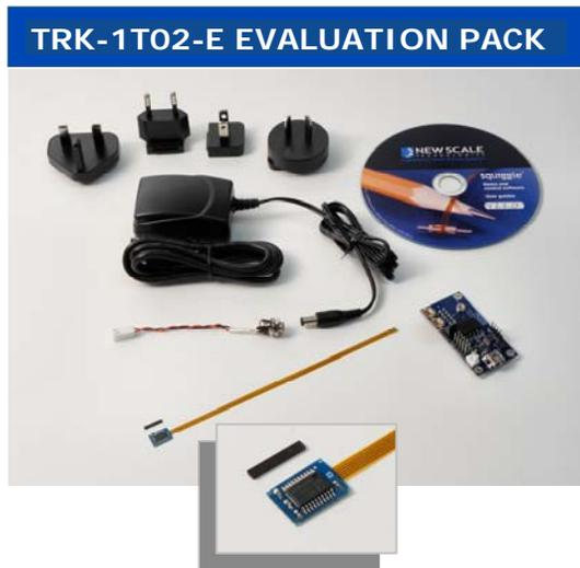
The TRK-1T02-E Evaluation Pack is a full-featured development platform for the NSE5310 Position Sensor. The MC-33MB interface card accepts the I<sup>2</sup>C input from one or two NSE5310 sensors, and connects via USB to your PC. Use the New Scale Pathway™ Software to view and collect position information. This development kit provides for easy sensor evaluation and system development.
